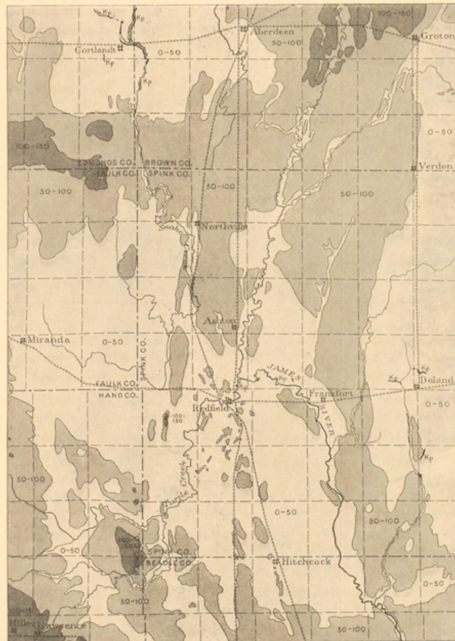
FIGURE 5.—Map of Northville, Aberdeen, Redfield, and Byron quadrangles showing approximate depth to base of the glacial till. Water can frequently be had from sands at the base of the till, and generally rises many feet in wells.
