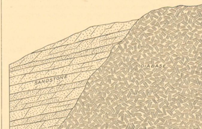
FIG. 6.—Upper contact of Palisade diabase in West Shore Railroad cut east of New Durham, N. J. Looking north. Shows dike-like attitude of west side of diabase cutting across Newark strata.
