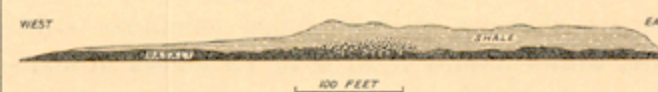
FIG. 3.—Section showing relations of surface of first Watchung basalt and its contact with overlying strata along south side of gorge northeast of Scotch Plains, N. J. Looking south.
