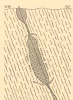
FIG. 25.—Cross section of the ore shoots along line A-A, fig. 23. The pods are known as shoots and the comparatively barren rock between them as pinches. The rock overlying the shoots—that is, that under which the ore
