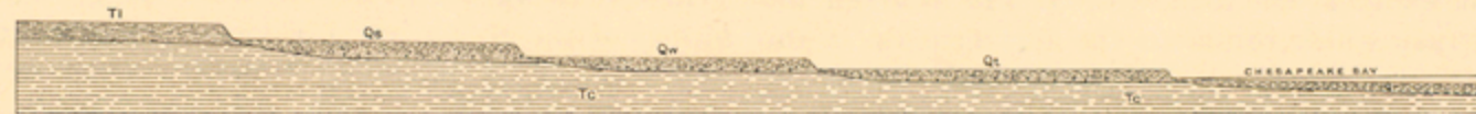
Fig. 2.—Ideal section showing structure and topographic relations of the several terrace formations. Qr, Recent; Qt, Talbot; Qw, Wicomico; Qs, Sunderland; Tl, Lafayette; Tc, Chesapeake group.
