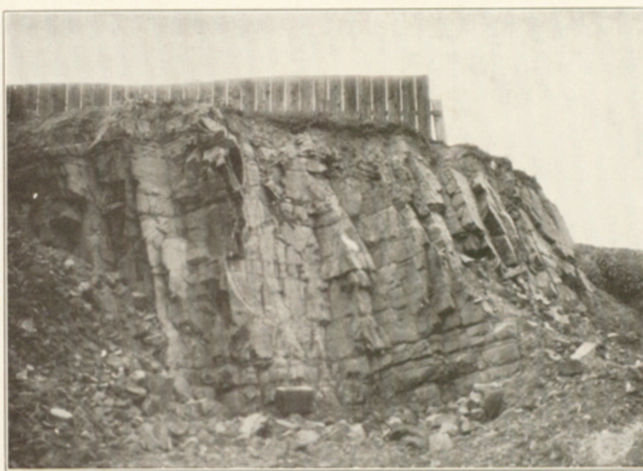
PLATE 5.—POROUS SANDSTONE RESIDUAL FROM SANDY CONESTOGA LIMESTONE AT McSHERRYSTOWN Crumbles to rounded sand grains and is quarried for building sand
