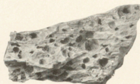
PLATE 37.—WEATHERED AMYGDALOIDAL GREENSTONE, FROM PIGEON HILLS, 1 1/2 MILES NORTHEAST OF BITTINGER The brown-weathered rock is pitted with round holes from which the filling, probably calcite, has been dissolved
