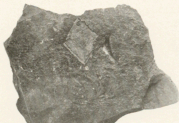
PLATE 22.—MOLD OF A LOZENGE-SHAPED CRYSTAL OF GLAUBERITE FROM A POINT NEAR GOLDENVILLE
