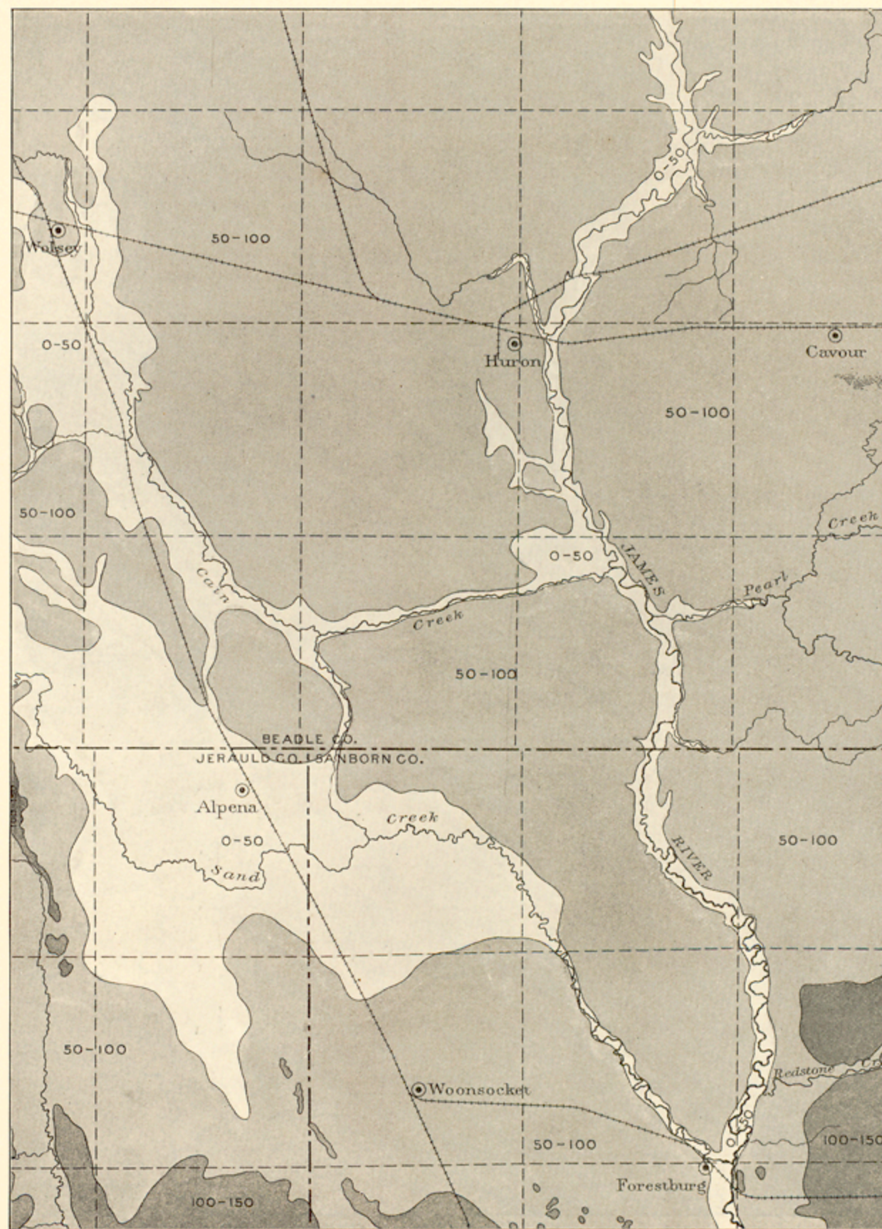
FIG. 7.—Sketch map of Huron quadrangle showing approximate depths to the bottom of the till. Water can usually be obtained from sands and gravel at the base of the drift, and generally rises many feet in wells.
