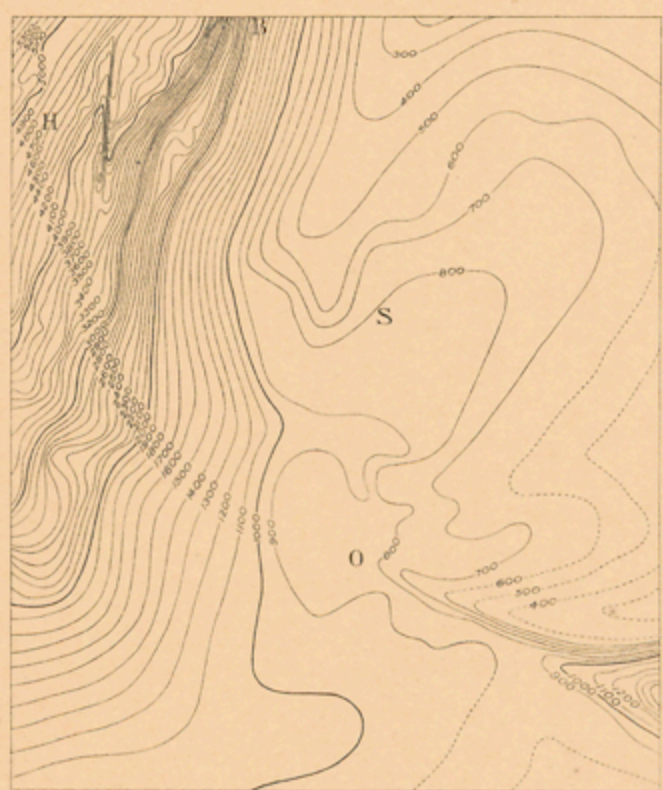
FIG. 1.—Diagram showing contour of surface of Dakota sandstone in the Oelrichs quadrangle. The lines represent altitudes above sea level and are 100 feet apart vertically. O, Oelrichs; S, Smithwick; H, Hot Springs; B, Buffalo Gap.
