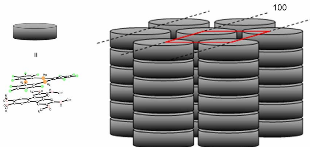
Figure 7.9. Cartoon depicting the proposed simple hexagonal cell used for indexing the powder patterns.
