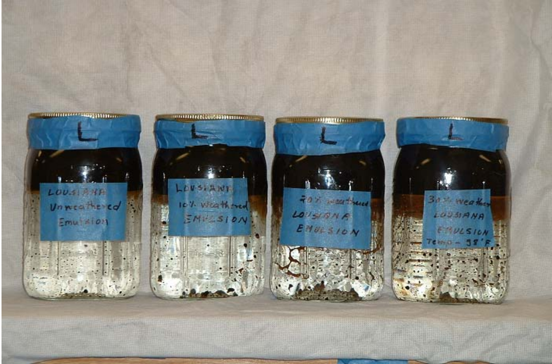
Fig. 16. Louisiana crude oil emulsions prepared by using mixing chamber for 24 hrs, reflect the correlation between the evaporation rate and the stability of the emulsions.
