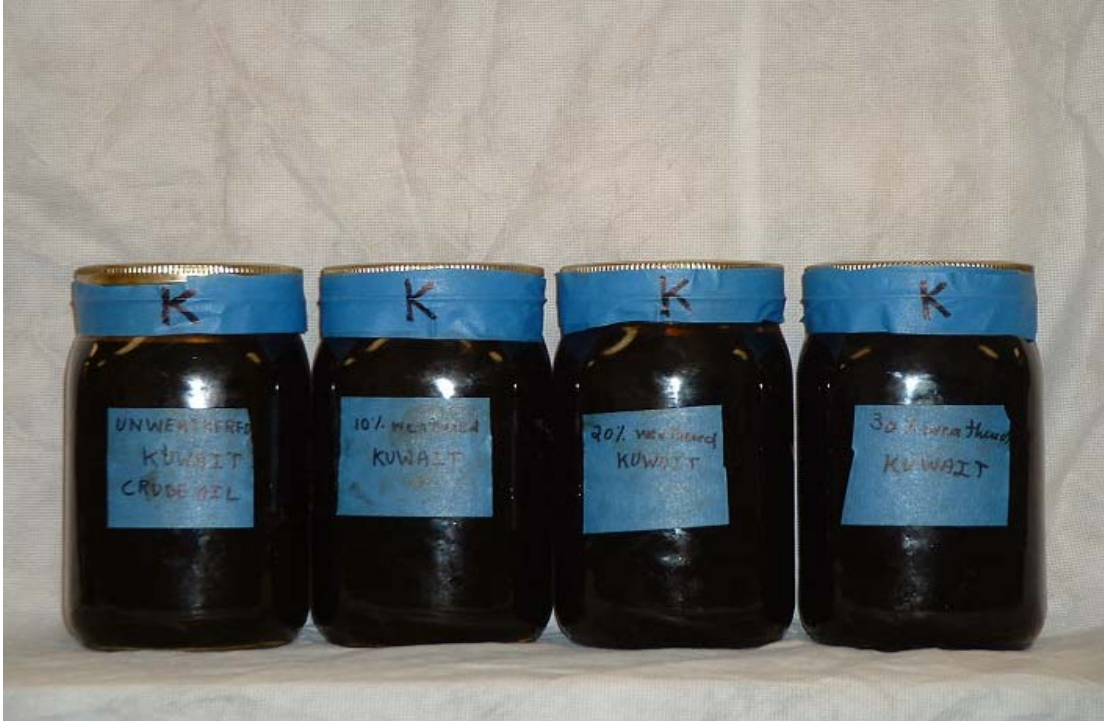
Fig. 10. Samples of un-weathered, 10% evaporated, 20% evaporated and 30% evaporated Kuwait crude oil. (From left to right)
