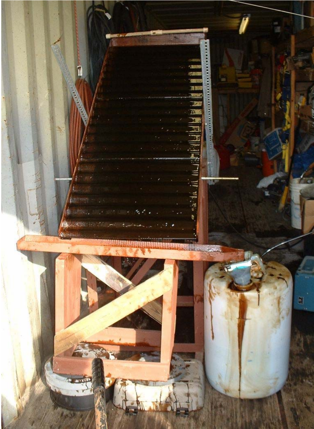
Fig. 3. Experimental setup for spreading and evaporation of the crude oil.
