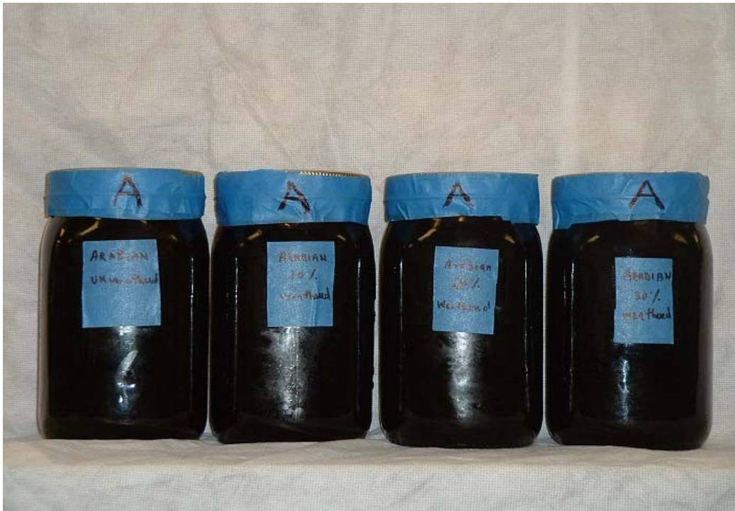
Fig. 9. Samples of un-weathered, 10% evaporated, 20% evaporated and 30% evaporated Arabian medium crude oil. (From left to right)
