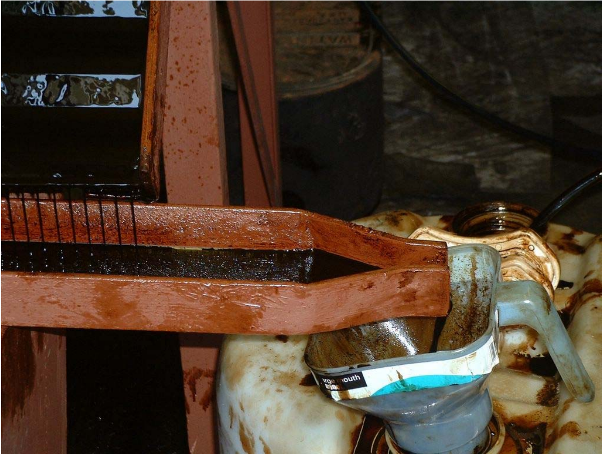
Fig. 7. Arrangement made to collect the crude oil coming from the corrugated plate.
