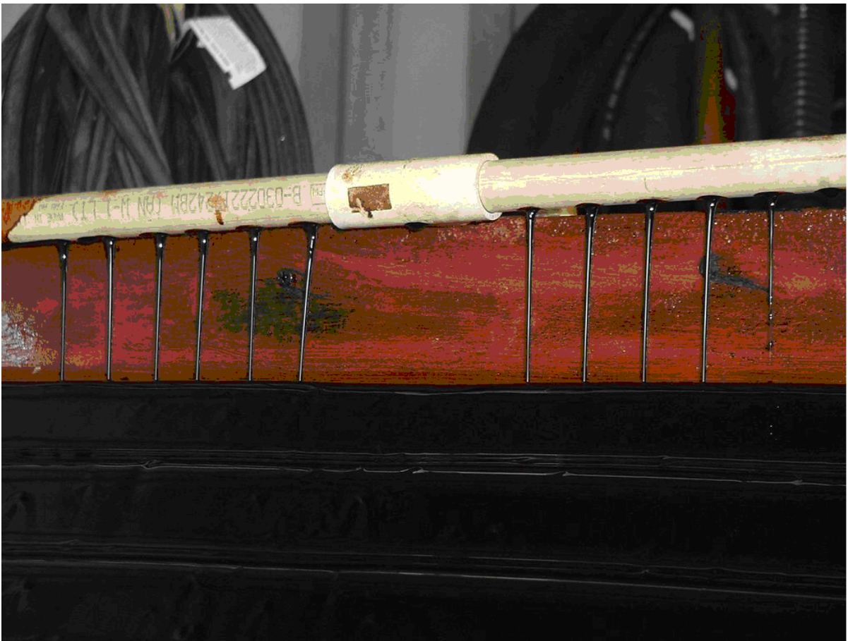
Fig. 6. Spreading device mounted at the top of corrugated plate
