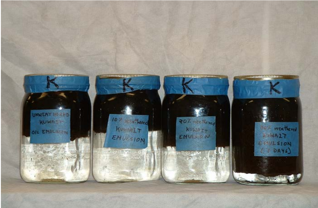
Fig. 14. Kuwait crude oil emulsions prepared by using mixing chamber for 24 hrs reflect the correlation between the evaporation rate and the stability of the emulsions.
