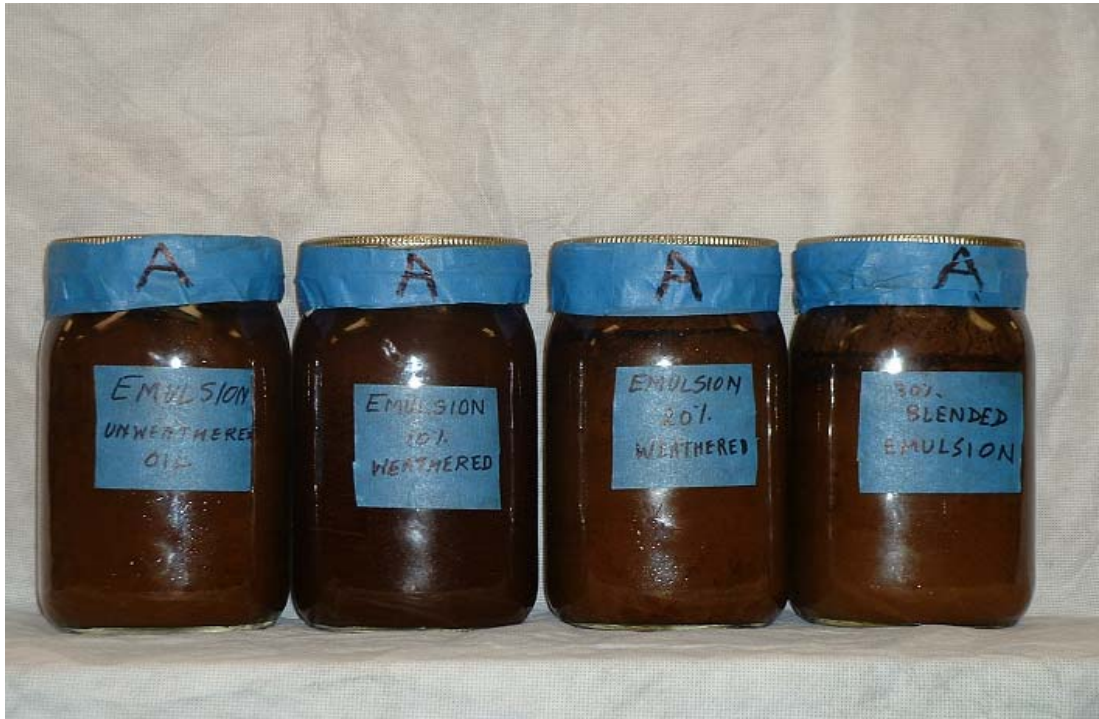
Fig. 13. Arabian medium crude oil emulsions (chocolate mousse) prepared by using regular blender
