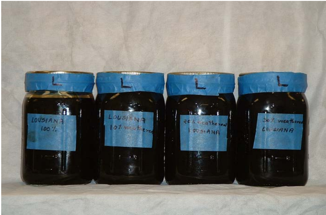
Fig. 11. Samples of un-weathered, 10% evaporated, 20% evaporated and 30% evaporated Louisiana crude oil. (From left to right)
