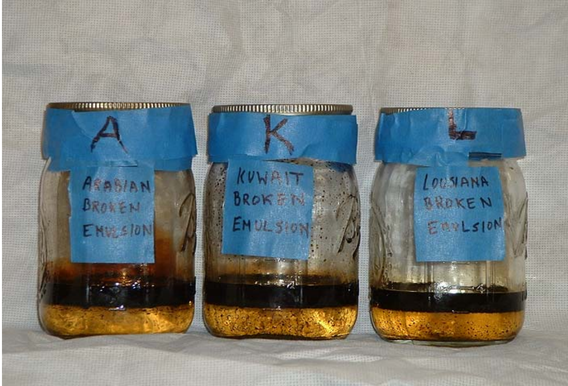
Fig 18. Oil water separation by addition of emulsion breaker EC2003A
