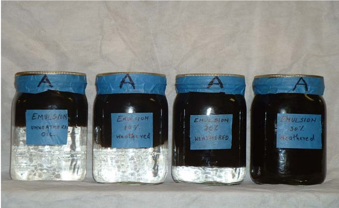
Fig. 12. Arabian medium crude oil emulsions prepared by using mixing chamber for 24 hrs reflect correlation between the evaporation rate and the stability of the emulsions.
