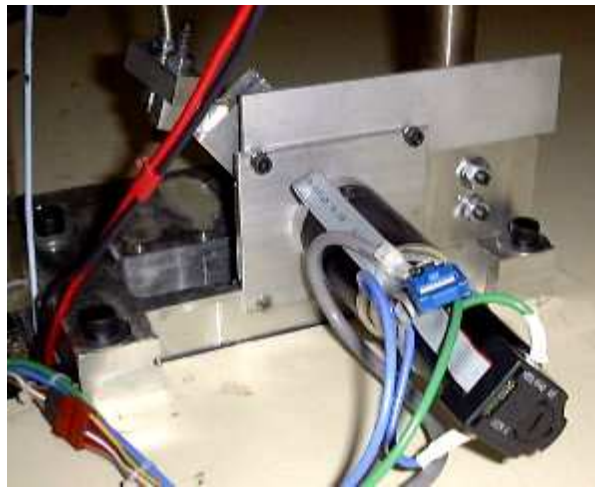
Fig. 8. DC Motor-linkage assembly for AOA control.
