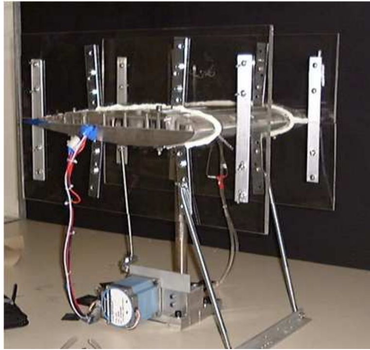
(a) NACA 0015 airfoil model embedding the synthetic jet actuator.
