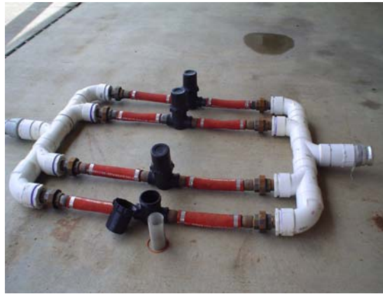
Figure 8. In-line water filter for rainfall simulator.
