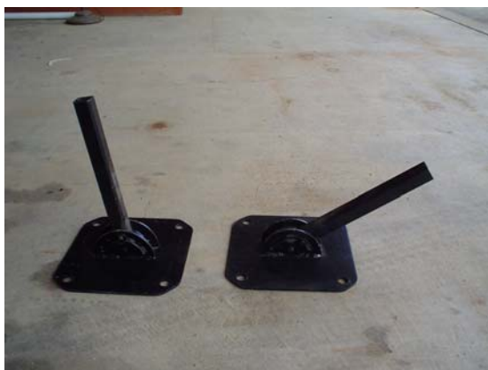
Figure 6. Rotating base plates used to support the rainfall simulation mast, set at differing angles.
