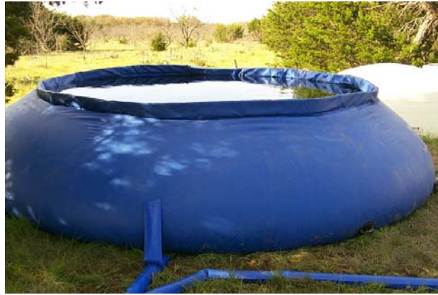
Figure 9. The 19,000 L portable collapsible water tank deployed at the research site.
