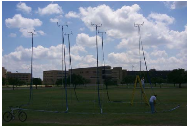
Figure 5. Image of completed rainfall simulator with masts supporting the sprinkler assemblies.
