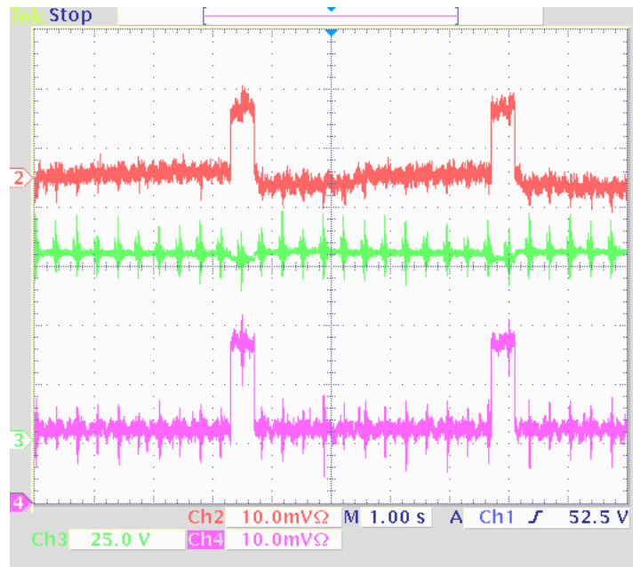
Fig. 55. Output voltage, battery current and output current with ultracapacitor as the auxiliary device.
