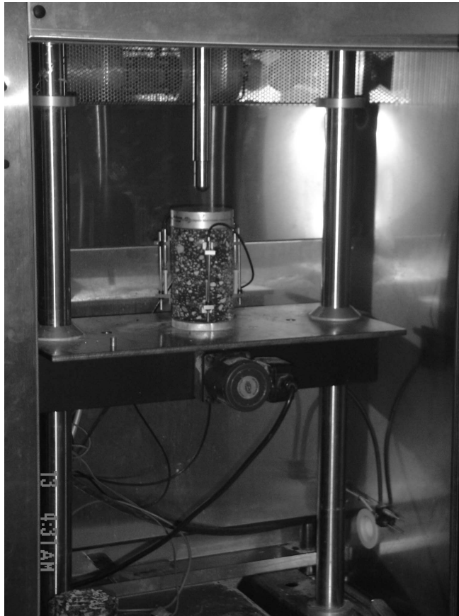
Fig. 9. MTS machine with temperature chamber removed
