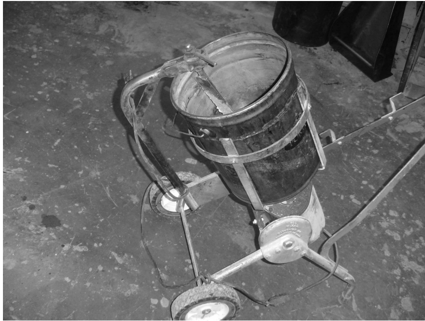
Fig. 2. Mechanical mixer for mixing asphalt and the aggregates
