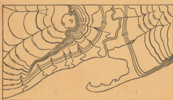
Fig. 1. The upper figure represents a sketch of a river valley, with terraces, and of a high hill enclosed by a cliff. These features appear in the map beneath, the slopes and forms of the surface being shown by contours.
