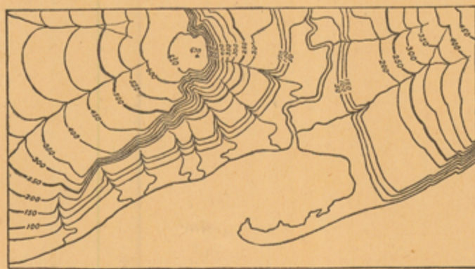
Fig. 1. The upper figure represents a sketch of a river valley, with terraces, and of a high hill encircled by a cliff. These features appear in the map beneath, the slopes and forms of the surface being shown by contours.
