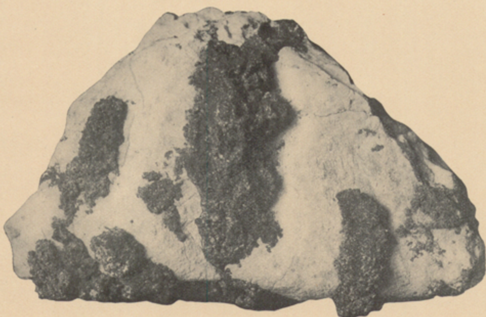
PLATE X.—MAGNETITE IN LIMESTONE OF HASMARK FORMATION IN CONTACT ZONE OF CABLE STOCK. The light-colored mineral mixed with the magnetite is iron-poor olivine, partly serpentinized.
