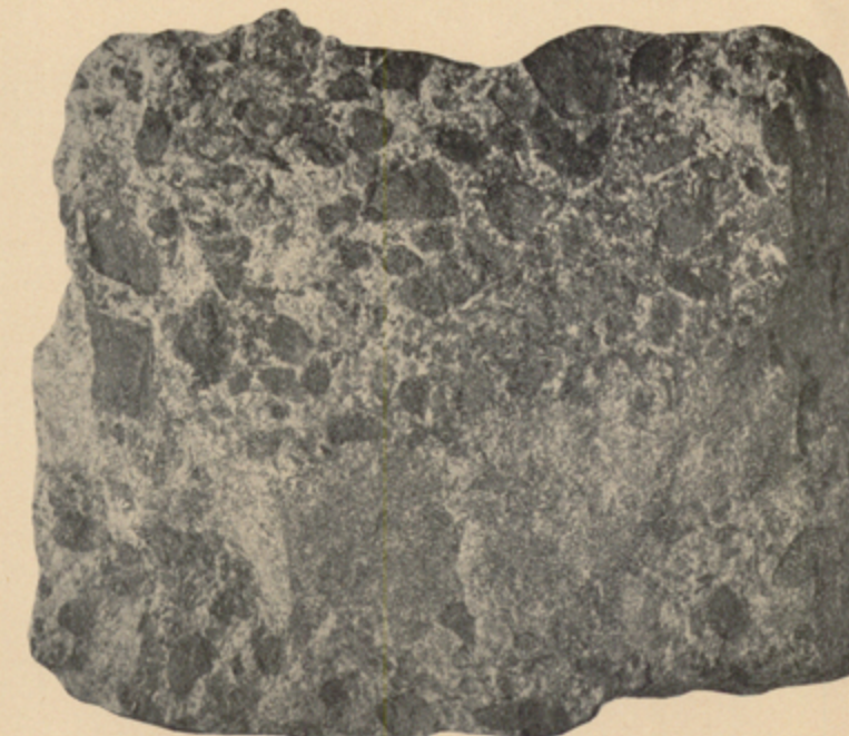
PLATE XII.—MUD FLAKES IN SPOKANE SANDSTONE. Angular and rounded fragments of dark-red argillite included as pebbles in the sandstone.
