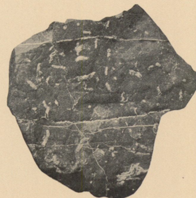
PLATE IX.—MAGNESIAN LIMESTONE OF LOWER PART OF HASMARK FORMATION. The roughness of the weathered surface is caused by projecting crystals of dolomite, which are less soluble than the calcite. The characteristic white tubular bodies are possibly fossil worm cases.
