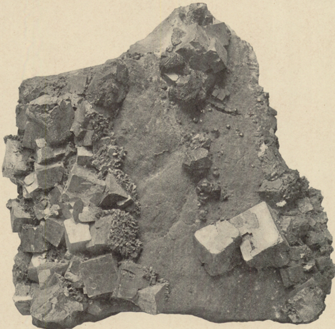
FIG. 22.—ZINC BLENDE AND COARSE GALENA CRYSTALS COVERED BY MARCASITE FROM CAVITY IN SHEET GROUND.
