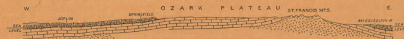
FIG. 2.—General west-east section through Joplin and the St. Francis Mountains. Showing the flat-topped dome of Cambrian and Ordovician limestones and pre-Cambrian crystalline rocks overlain by thin Devonian shale and Carboniferous sediments.
