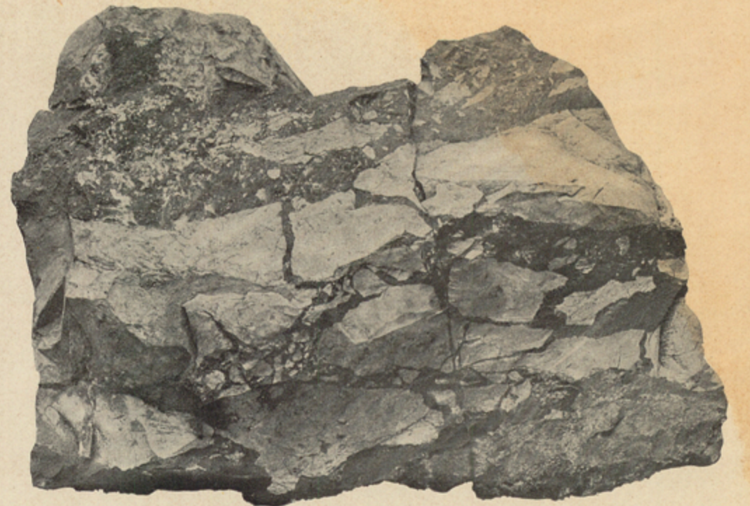
FIG. 16.—ZONAL CHERT BRECCIA WITH JASPEROID CEMENT. The angular chert fragments are parts of one mass but little displaced.
