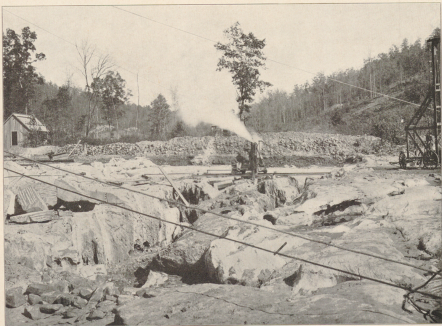
FIG. 2.—SURFACE OF MURPHY MARBLE, STRIPPED FOR QUARRYING; 2 MILES SOUTHWEST OF TOMOTLA. LOOKING NORTHEAST ALONG THE STRIKE. Beyond the quarry is seen a thin layer of auriferous gravel, which has elsewhere been successfully washed for gold. On the right is a ridge of Nottely quartzite; on the left a ridge of Valleytown formation.
