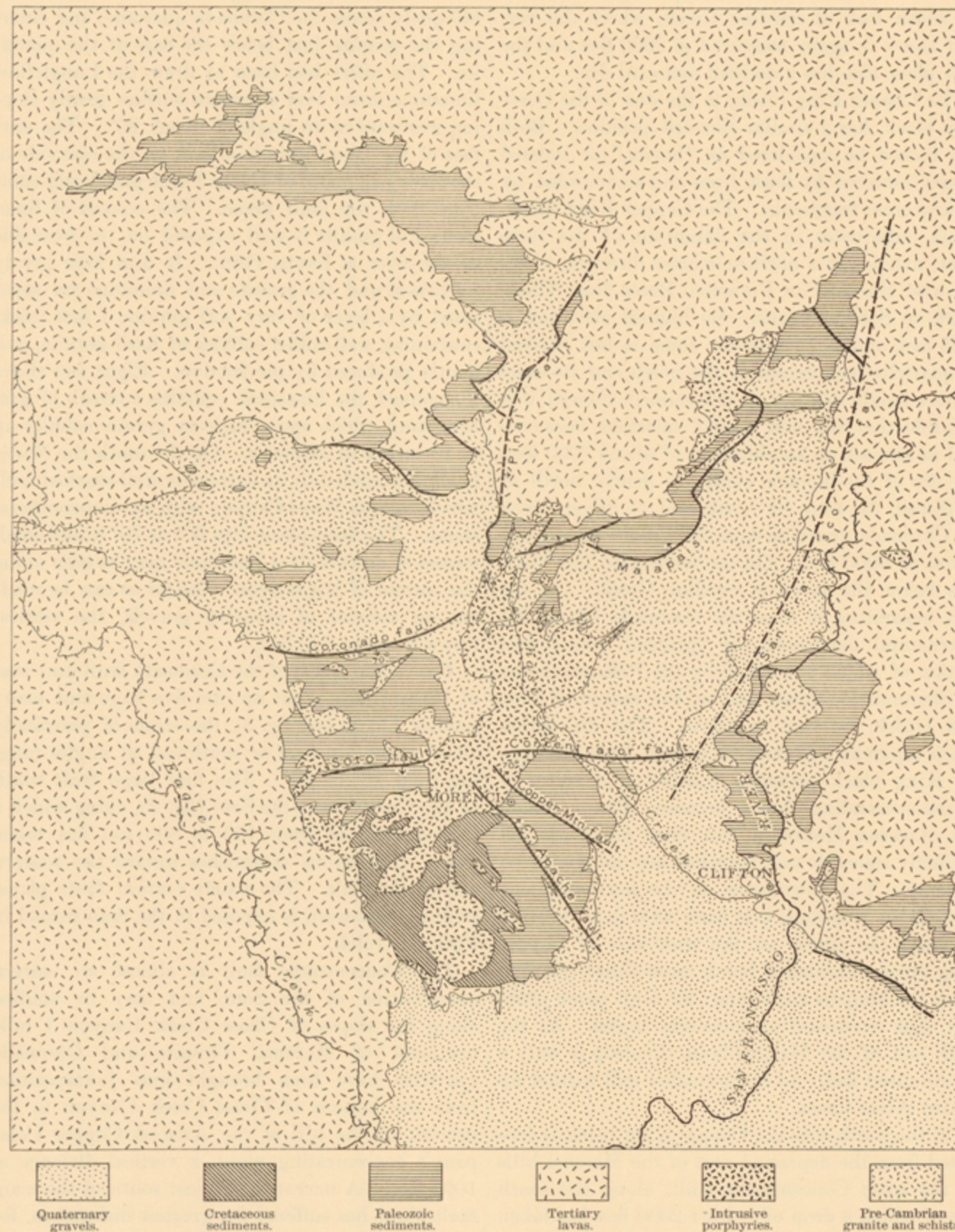
FIG. 2.—Generalized geologic map of Clifton quadrangle, showing the major faults. Arrows show dip and downthrown side of faults. Scale, approximately, 1 inch=2 miles.
