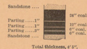
FIG. 3.—Section of coal near conduit of Marshfield waterworks.
