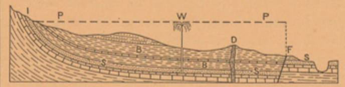
FIG. 3.—Ideal section showing artesian conditions where the outflow is obstructed by faulting. SS, water-bearing stratum. BB, impermeable bed. D, dike. F, fault. W, well. I, inflow. PP, plane of head.
