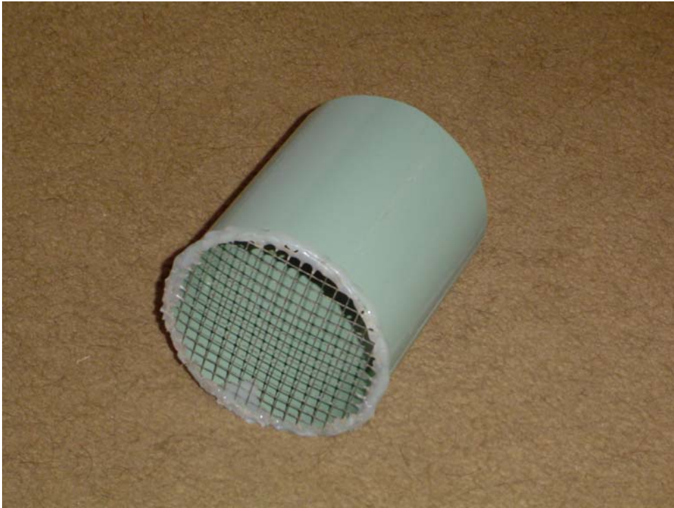
Figure 2. Termite bait trap (10 cm diameter, 12.5 cm height) with mesh (0.6 cm x 0.6 cm openings) bottom exposed.
