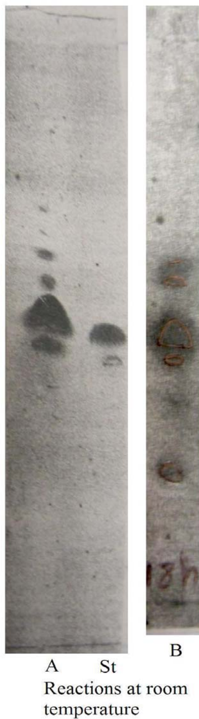
Figure II-11. Removal of the TBDMSi group with TBAF/HF/MeMo (A) and with \text{BF}_3 (B). The HDA- \beta CD standard is shown on lane St. The silica TLC plates were run with an eluent 50:10:1 \text{CHCl}_3 :MeOH: \text{H}_2\text{O} .
