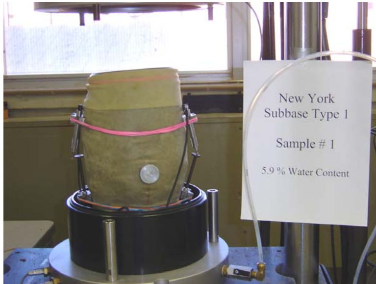
FIGURE 34 Type 1 specimen #1 at 5.9 % water content at the end of testing.
