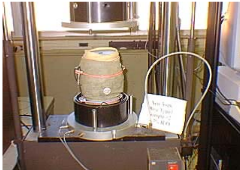
FIGURE 35 Type 1 specimen # 2 at 4.3 % water content at the end of testing.
