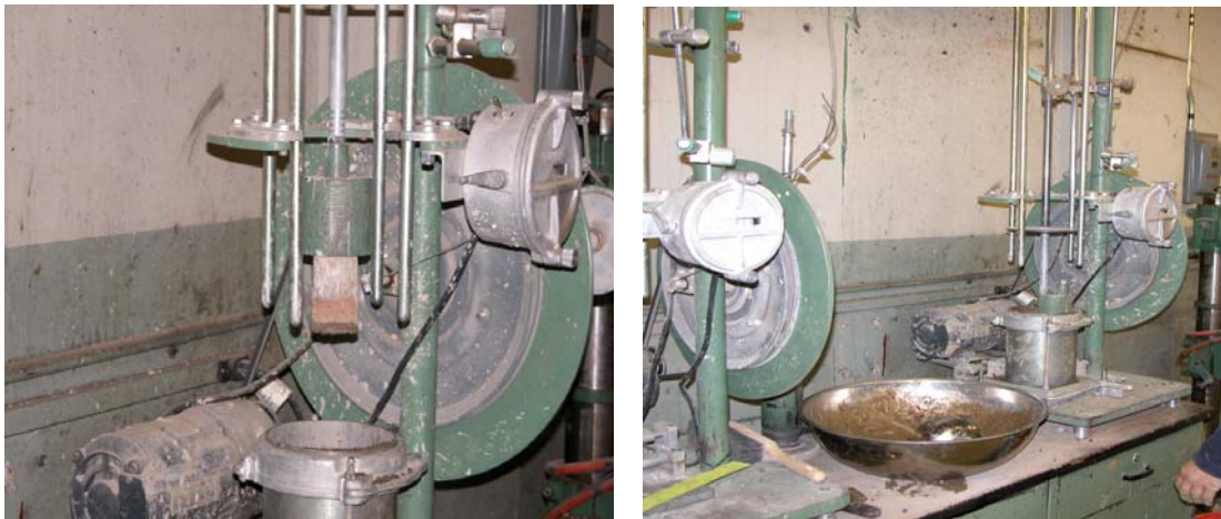
FIGURE 7 Molding and compacting equipment.
