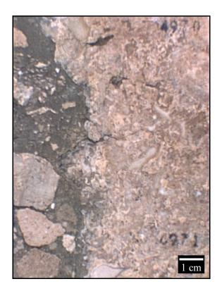
Figure 9. Core photo of *Tubiphytes* bindstones. Core sample is from 4971 feet, well Lott 19-4. The bindstone, or reefy material is located in the right portion of the photo adjacent to floatstone clasts.
