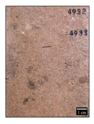
Figure 6. Core photo of oolitic grainstone at 4933 feet, well Lott 19-4. Note well developed skeletal-moldic porosity.
