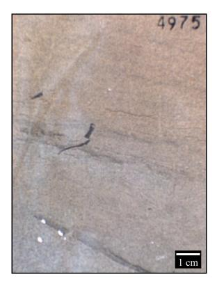
Figure 10. Core photo of siliciclastics. Core sample is from 4975 feet, well Lott 19-4. Note wavy ripples (black) near center of photo.
