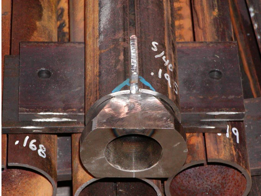
Figure 22. Expanding Tube Mandrel Placed Inside 3-inch Pipe
