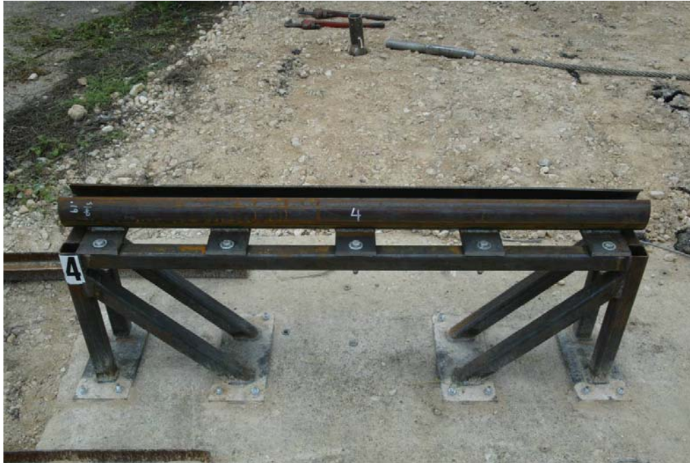
Figure 28. Pipe after Mandrel Has Traveled Through
