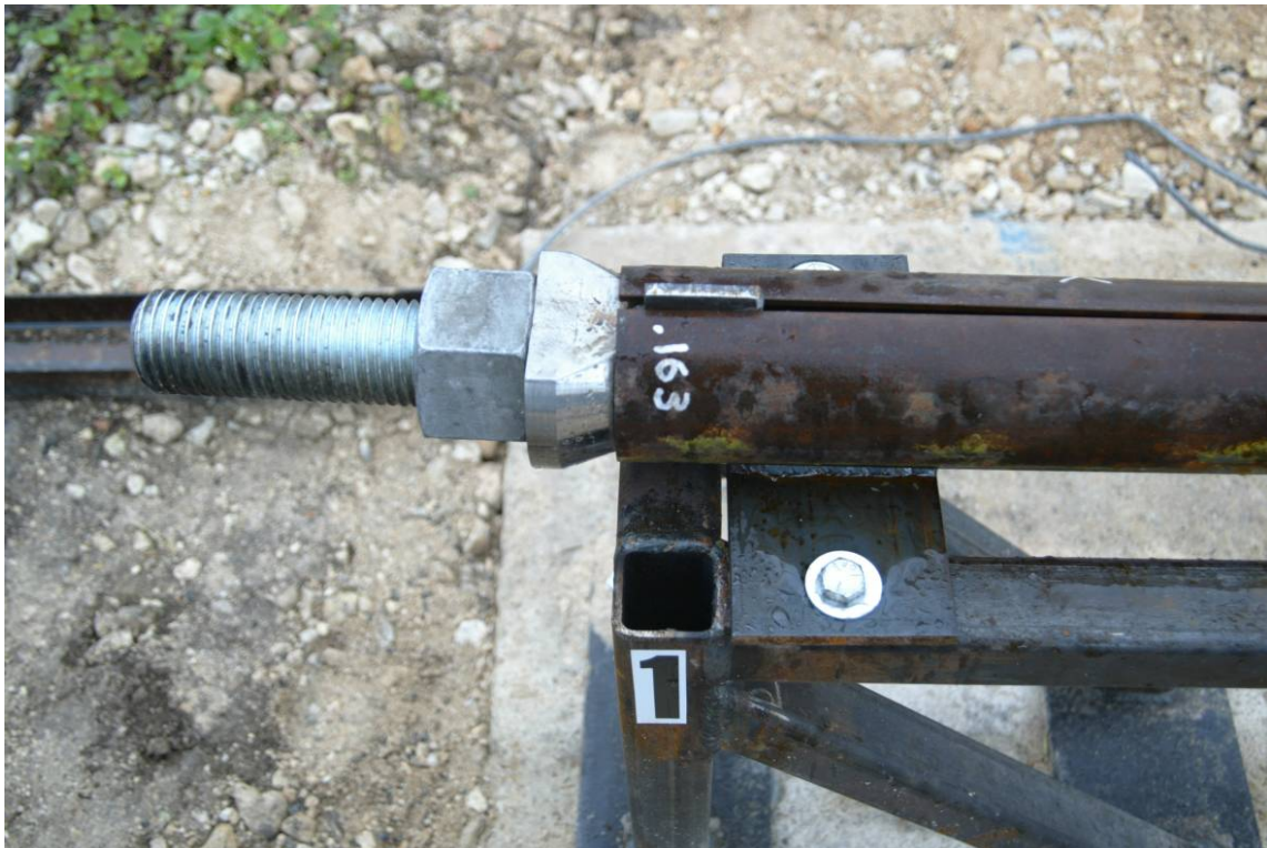
Figure 24. Nut Fastened to Threaded Swage
