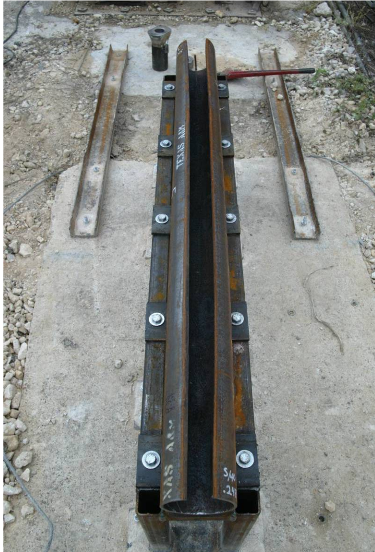
Figure 29. Deformed Pipe after Test
