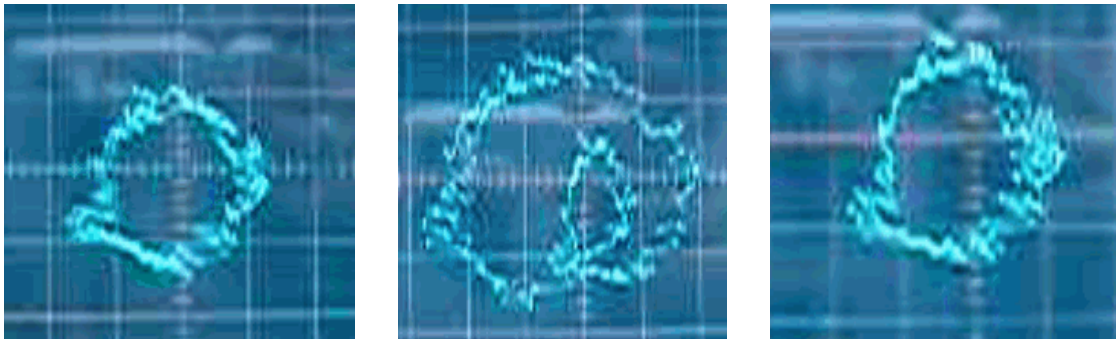
Fig 46: Orbits before, at and after the onset of subsynchronous vibration at twice the critical speed From an analog oscilloscope
