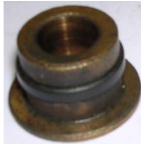
Fig 68: Worn-out sleeve bearing
