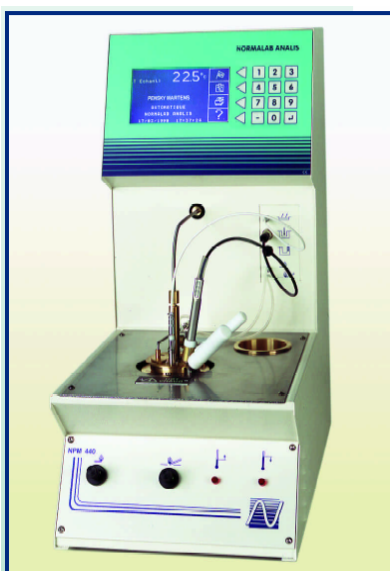
Figure 2. Closed cup tester used at PVAMU.
