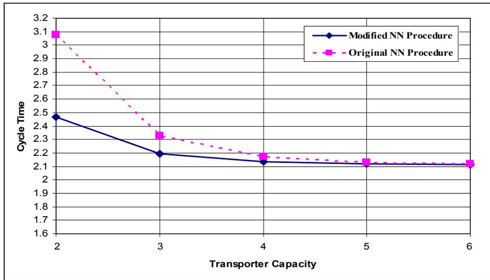
Figure 25. Plots for cycle times under both dispatching procedures for the example system with an outlier.
