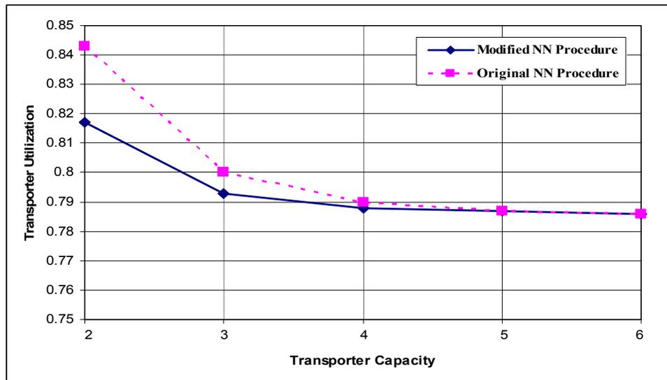
Figure 27. Plots for transporter utilizations under both dispatching procedures for the example system with an outlier.
