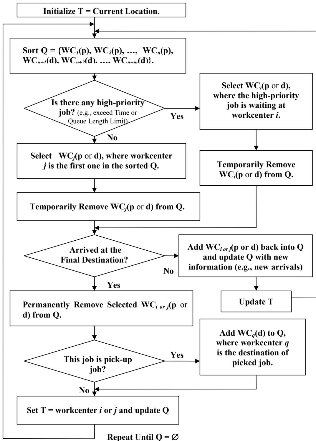
Figure 22. Flow diagram of the modified NN heuristic dispatching procedure.
