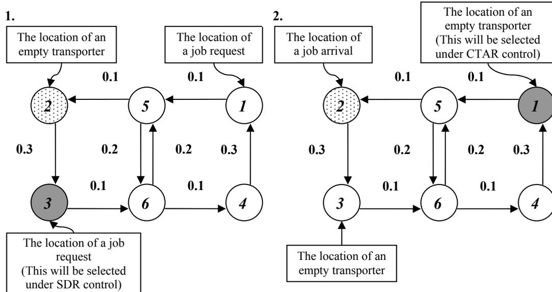
Figure 18. The difference between selection schemes under SDR control and under CTAR control for our unidirectional circuit network layout example.
