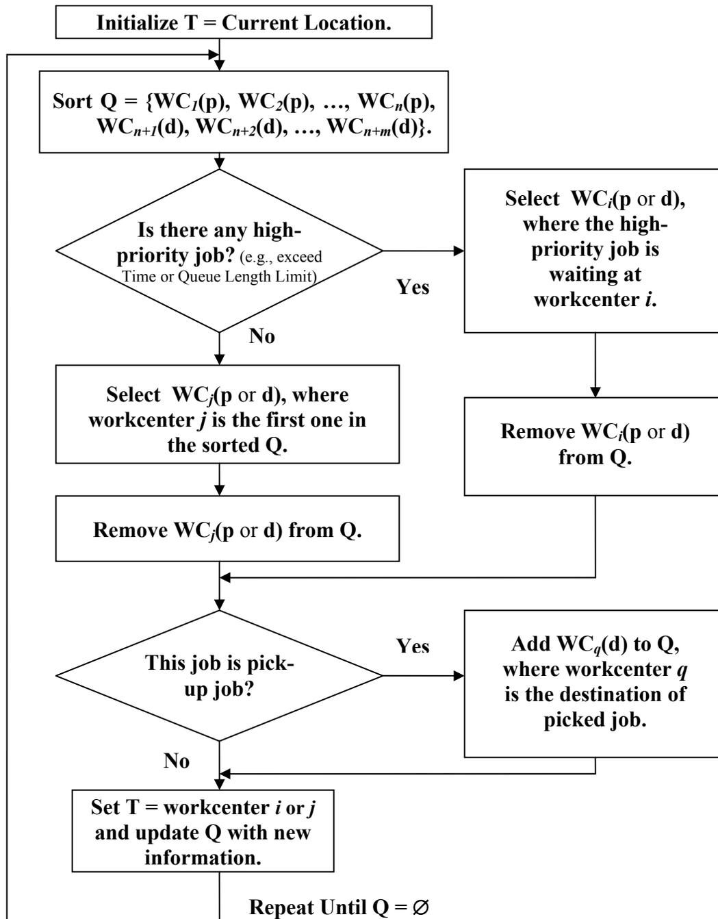
Figure 21. Flow diagram of the original NN heuristic dispatching procedure.
