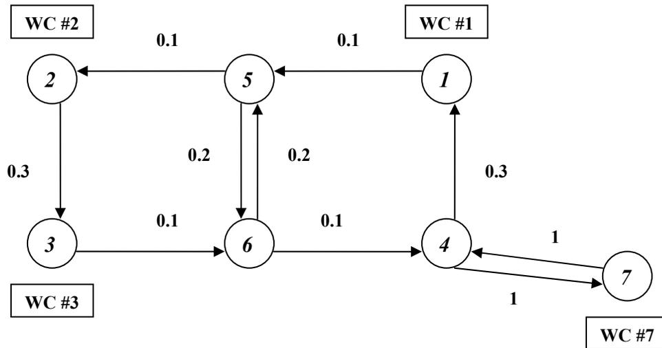
Figure 8. A fixed-route unidirectional material-handling system with an outlier (workcenter 7).
