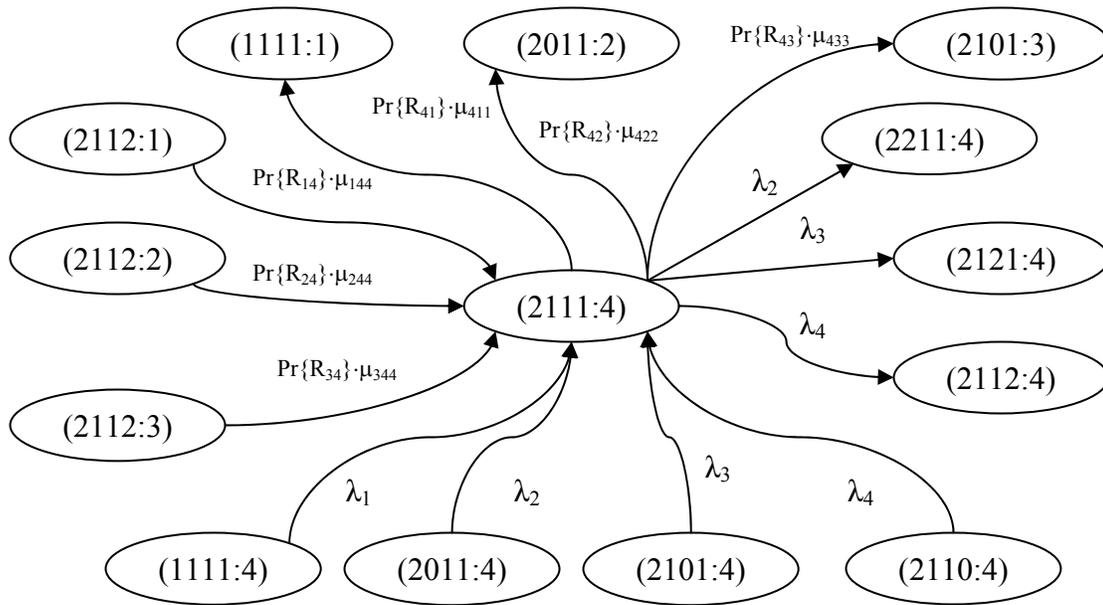
Figure 11. The diagram of all possible state transitions for state (2111:4).
