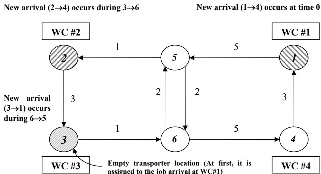
Figure 23. The example layout configuration for the fixed-route unidirectional material-handling system.
