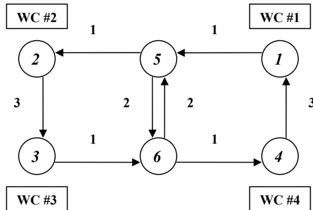
Figure 1. A fixed-route unidirectional material-handling system.
