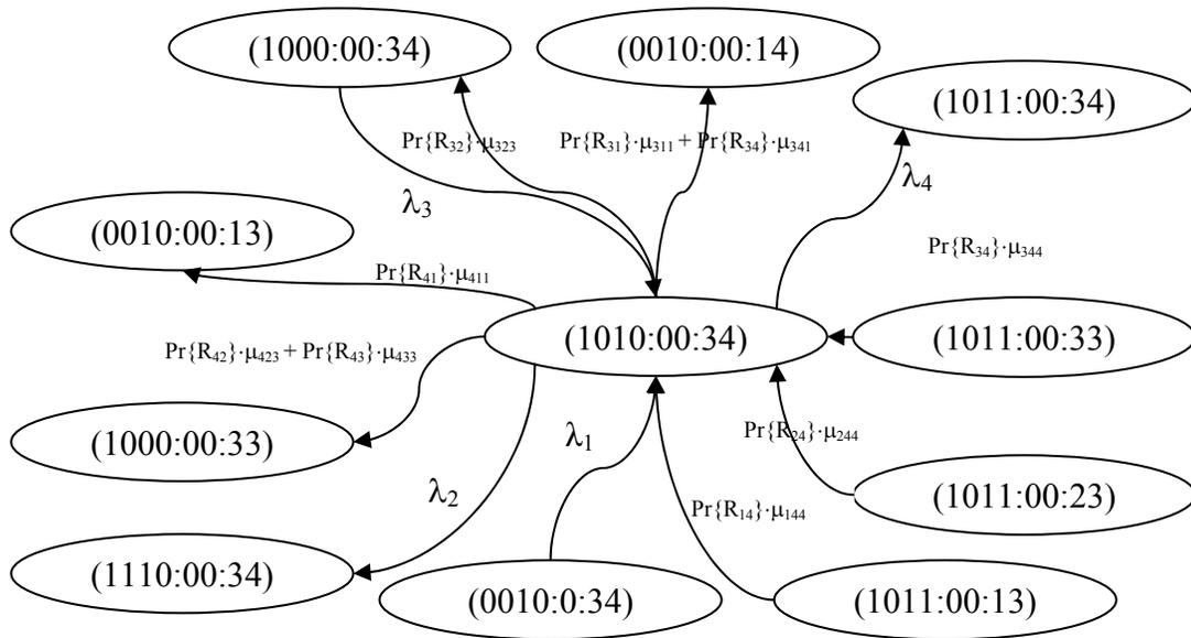
Figure 19. The diagram of all possible state transitions for state (1010:0:34).
