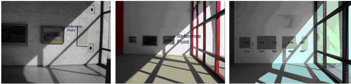
Figure A 2 Pictures of northeastern wall: the museum site (left), scale model (center), and Desktop RADIANCE model (right).
