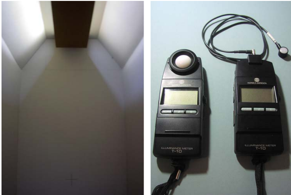
Figure 25 Interior view of scale model (left) and illuminance meters (Konica Minolta, T-10, right)
