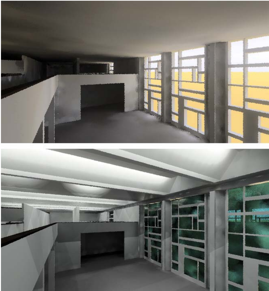
Figure B 4 Comparison between before (upper) and after (lower) installing top light side shading (Southeast gallery, 12:00 PM, Jun 21, Clear Sky)
