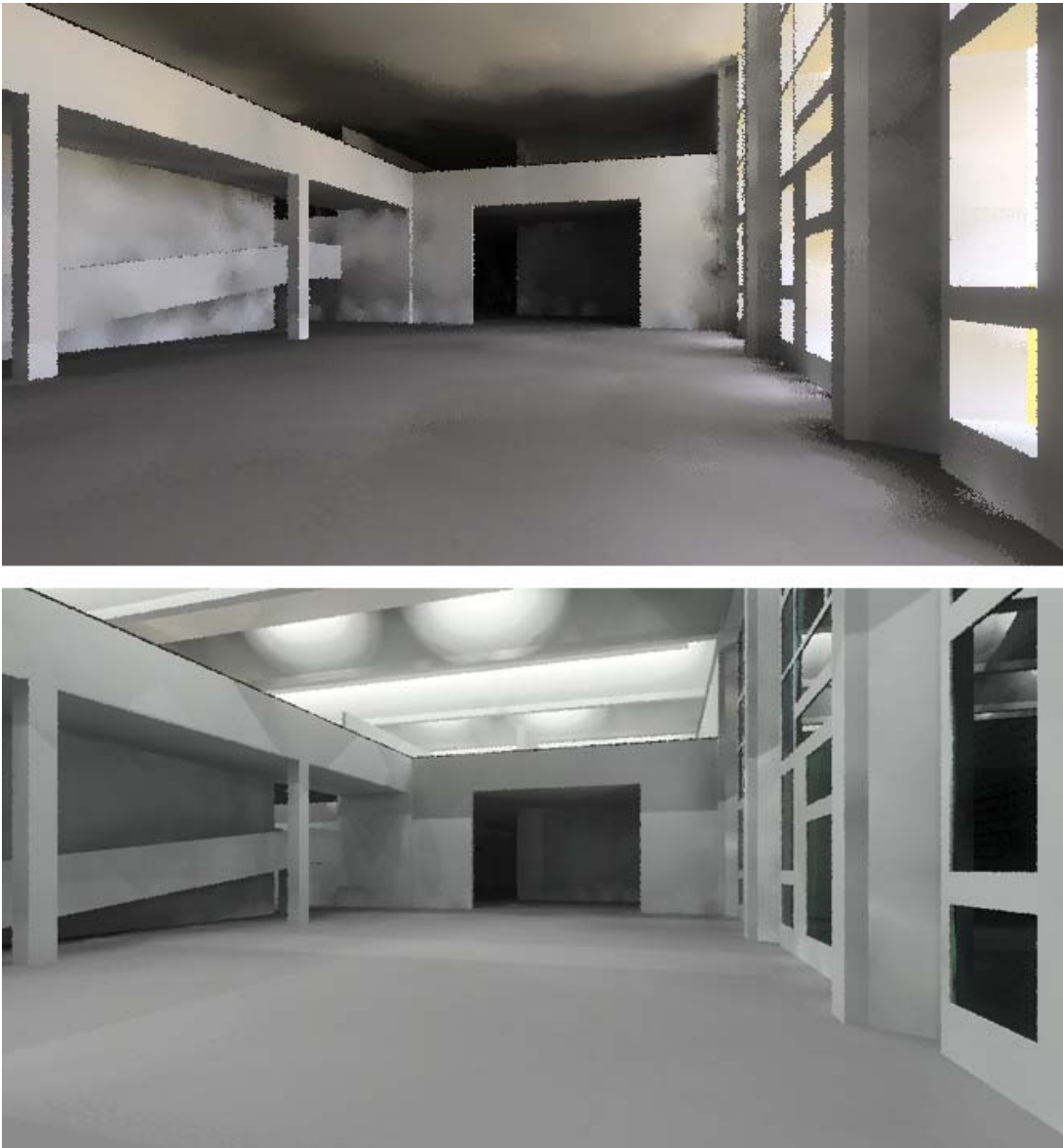
Figure 47 Comparison between before (upper) and after (lower) installing top light side shading (Southeast gallery, 12:00 PM, Jun 21, Clear Sky)
