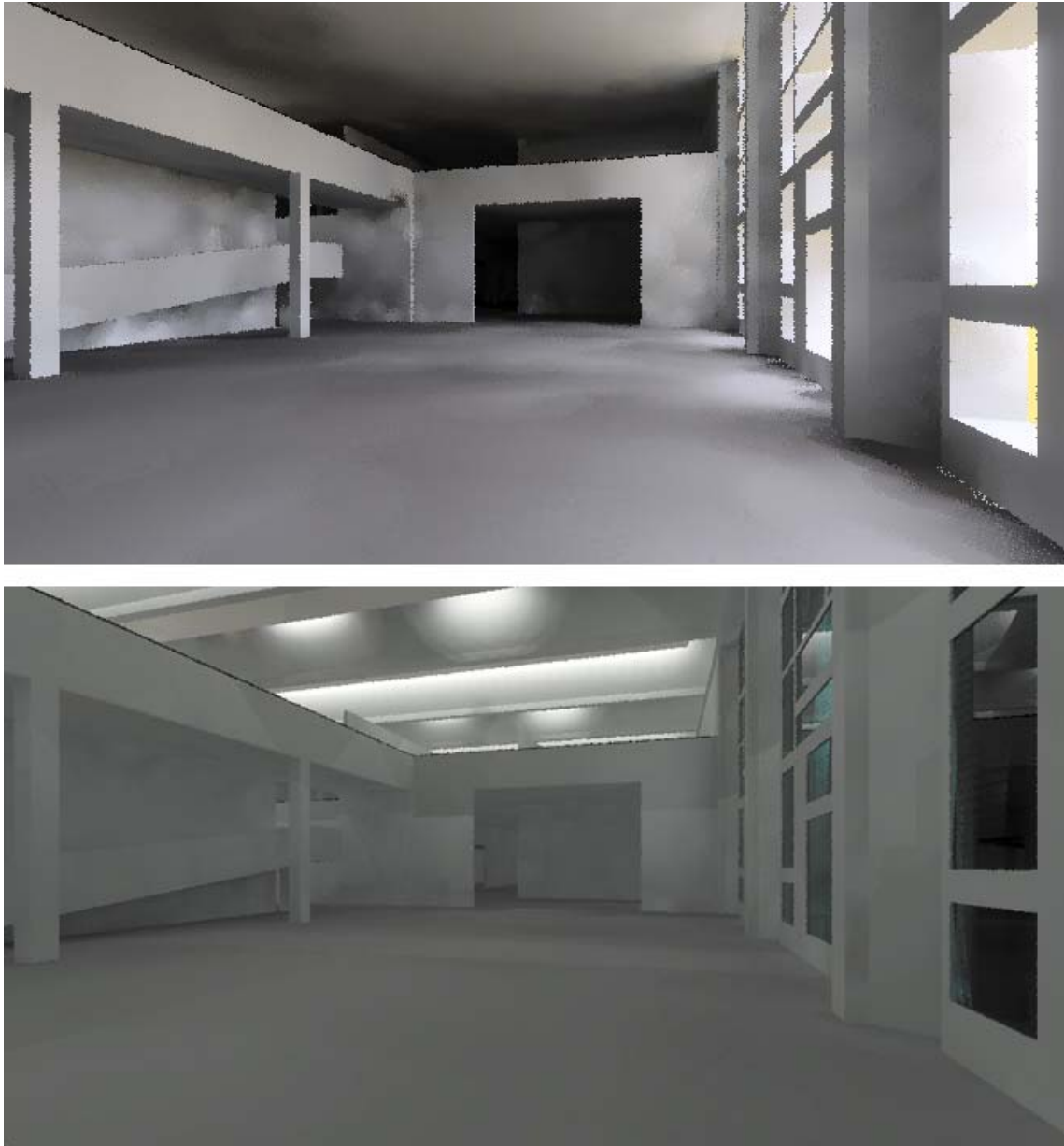
Figure B 1 Comparison between before (upper) and after (lower) installing top light side shading (Southeast gallery, 12:00 PM, Jun 21, Overcast Sky)
