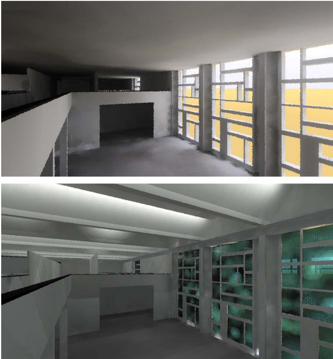
Figure B 5 Comparison between before (upper) and after (lower) installing top light side shading (Southeast gallery, 12:00 PM, Jun 21, Overcast Sky)
