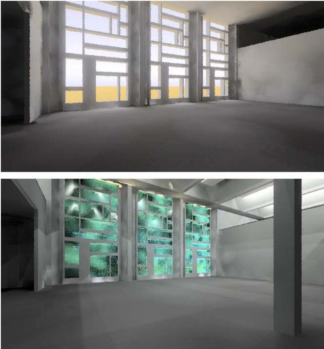
Figure B 2 Comparison between before (upper) and after (lower) installing top light side shading (Southeast gallery, 12:00 PM, Jun 21, Clear Sky)
