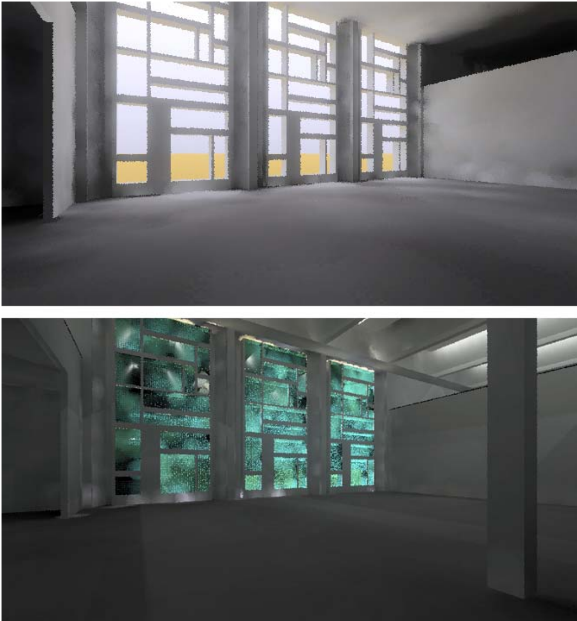
Figure B 3 Comparison between before (upper) and after (lower) installing top light side shading (Southeast gallery, 12:00 PM, Jun 21, Overcast Sky)
