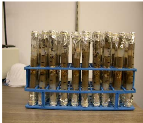
Figure 8. Bioassay design used to test the tunneling rate and mortality of both termite species when exposed to M. anisopliae grown on rice and corn.
