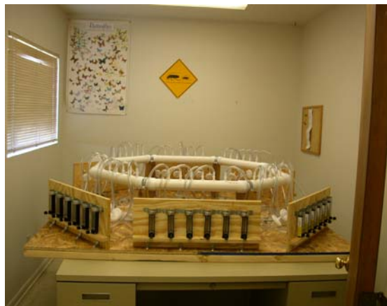
Figure 5. Olfactometer design used to determine the termites' preferences for volatiles produced by the M. anisopliae fungal strains.
