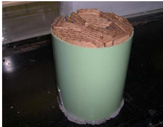
Figure 2. Reticulitermes flavipes trap made up of 12.5 X 10 cm PVC pipe filled with moistened strips of corrugated cardboard.
