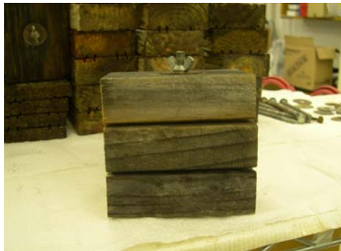
Figure 3. Coptotermes formosanus trap made up of three 12x12 cm wooden boards that were placed on a 14 cm long screw and secured at the end by a wing nut.
