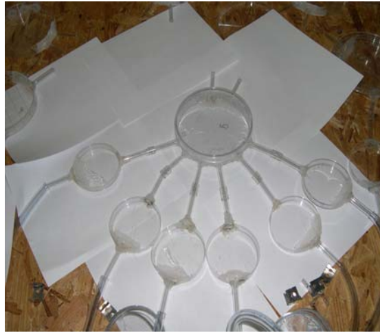
Figure 6. A view of one replication found in the olfactometer design that was made up of a center chamber and the six radiating dishes.
