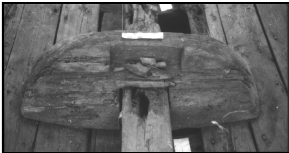
Figure 27: Main mast step, view aft. Photo by Christopher R. Sabick
