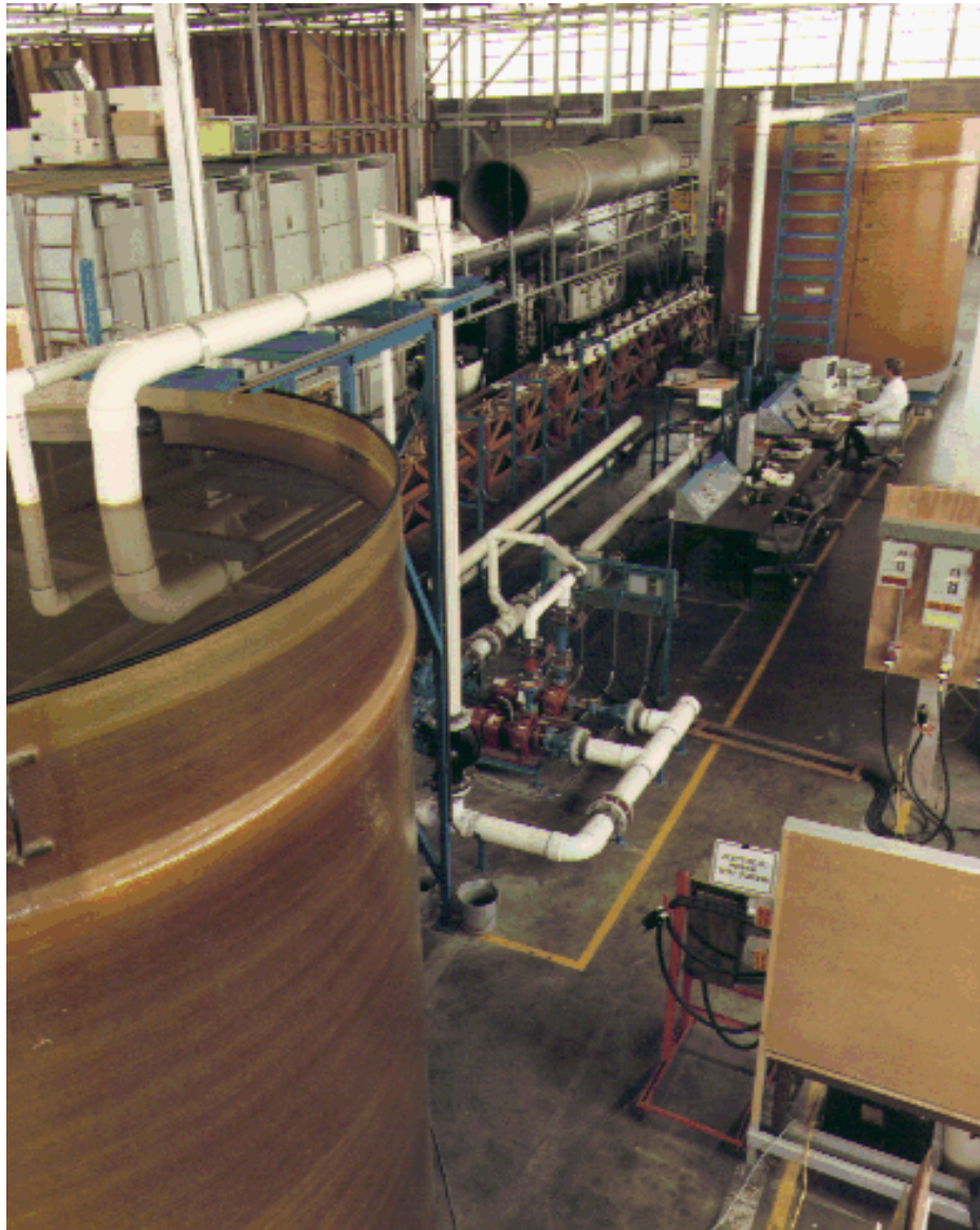
Figure 7: Photo of the ESL's Dynamic Weight Liquid Flow Loop. This flow loop measures flow rates using dynamic weight, as well as 2 nd and 3 rd reference standards (i.e., orifice plate, and magnetic meter). The flow loop is used to develop dynamic flow accuracies for flow meters in 3 to 12 inch diameter pipes, with flow rates varying from 50 to 650 gpm.
