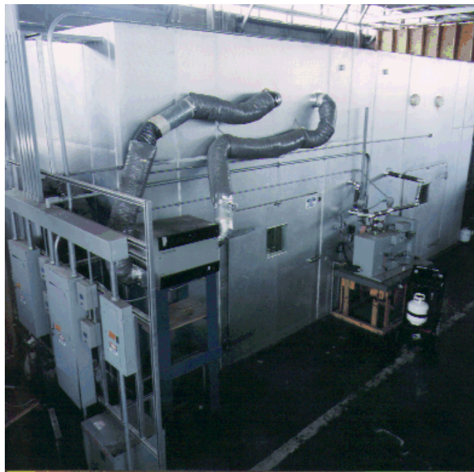
Figure 6: Photo of the ESL's Psychrometric Test Facility. This facility provides a controlled environment for testing unitary air conditioning and heat pump systems, +10^{\circ}\text{F} to +120^{\circ}\text{F} , and to measure relative humidity from 5% to 95%, with air flow rates from 150 CFM to more than 5,000 CFM in an AMCA flow chamber (ASHRAE Standards 116-83 and ARI 210/240-89).
