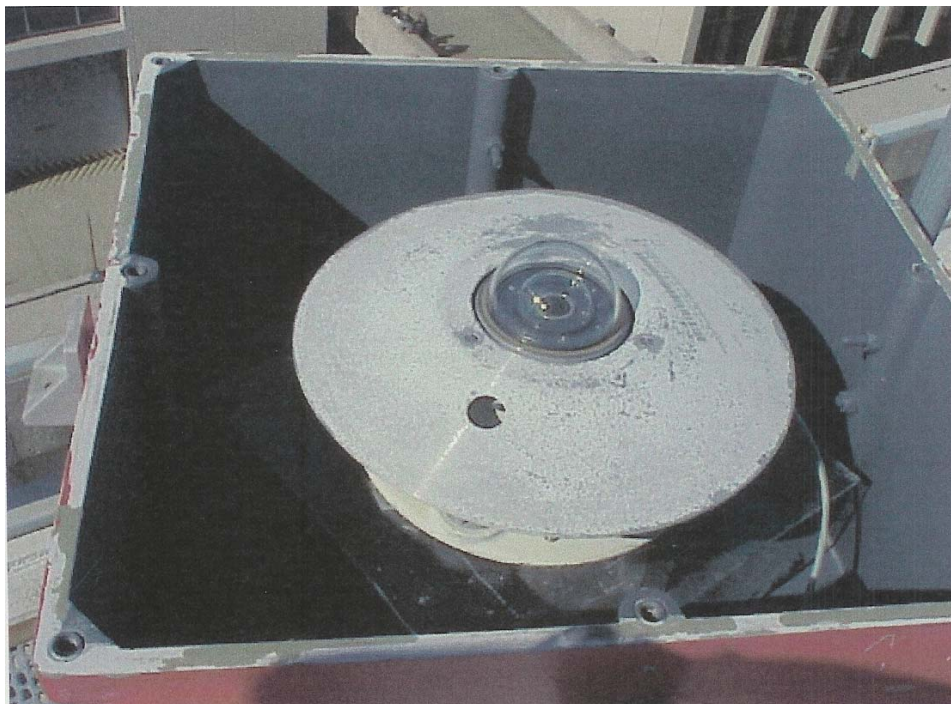
Figure 18: Close-up photo of transmittance test box.
