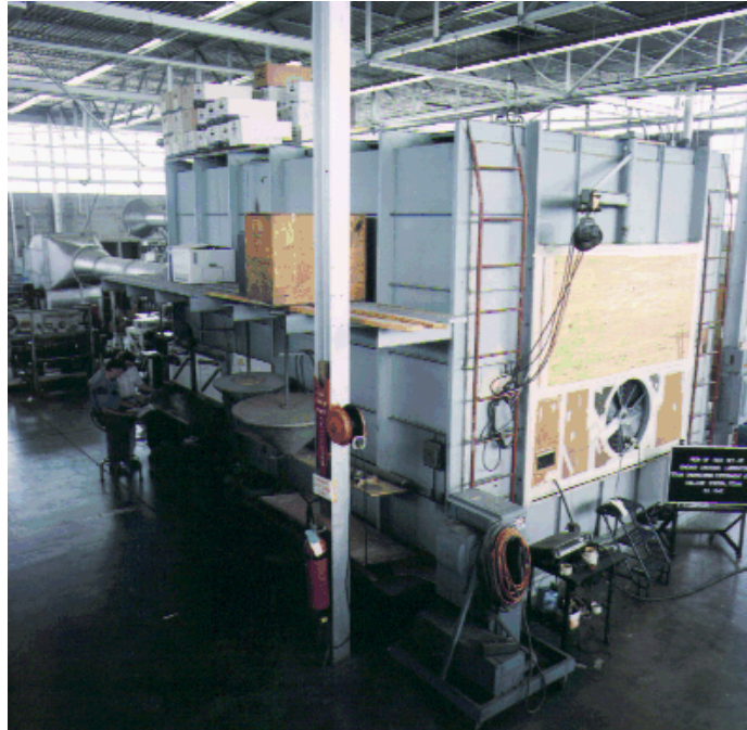
Figure 5: Photo of the ESL's Air Flow Chamber. This chamber is capable of measuring air flow as high as 50,000 CFM with accuracy of \pm 1\% , and can test fans with diameters of 8 ft, using ANSI/AMCA Standard 210-85.
