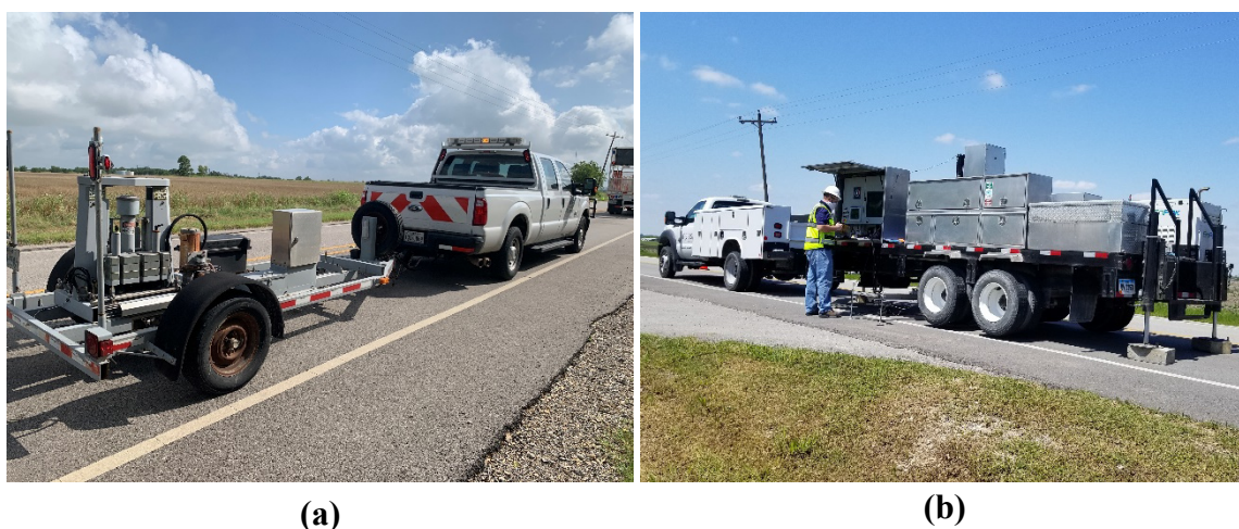
Figure 40 Nondestructive pavement testing: a) Falling weight deflectometer (FWD), and b) automated plate load test (APLT)
