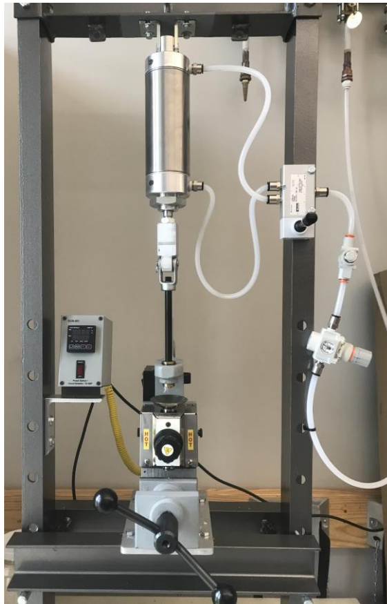
Figure III-3. Injection mold setup with pneumatically actuated barrel and temperature-controlled hopper.
