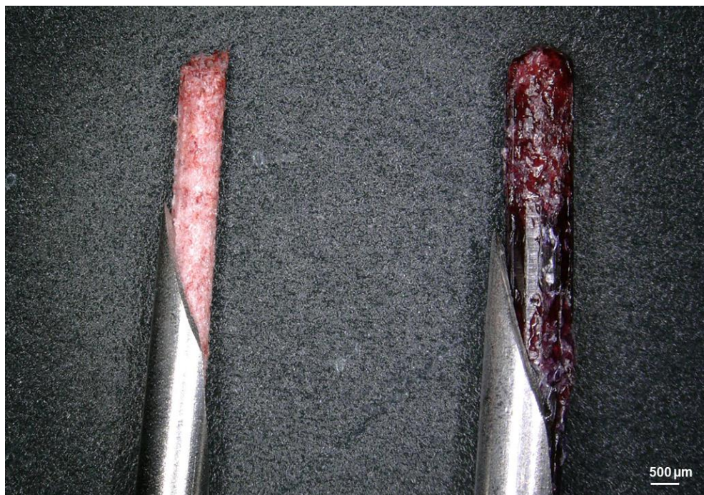
Figure IV-16. Keyence image of Dox-loaded SMP foams in needles for injection. The right-hand side shows a 0% PD foam that is loaded into an 18G needle. The left-hand side of this image shows the 10% PD foam that is loaded into a 16 1/2 G needle. In order for some procedures to be considered “non-invasive” it must be injected from a needle of 18 G (or higher gauge, smaller diameter). Our study design for the intended application in breast cancer does not necessitate injection, and this is just a proof of concept for future work where this may be desired.
