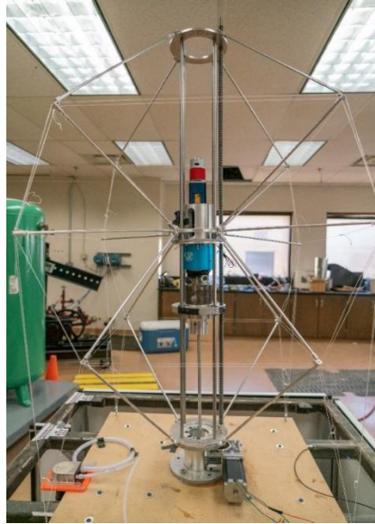
Figure 5.1. The Tensegrity Drilling Rig. We can see the tensegrity support structure holding the guide rods that support the Drill System shown in Figure 5.2 below.
