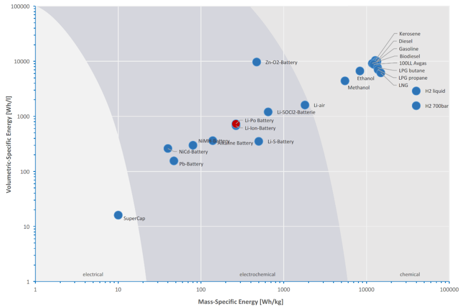
Figure 1.4 Volumetric-Specific energy Vs Mass-Specific energy. For various drone energy sources. The figure shows shaded zones for electrical, electrochemical, and chemical power sources for drones. Li-Po and Li-Ion are the most common sources for drones. Lithium-Thionyl-Chloride (Li-SOCL 2 ) and Lithium-Air have 2 times and 7 times higher energy density compared to Lithium Li-Po. Liquid Hydrogen has a much higher energy density at a factor of 150 times more energy density compared to Li-Po. Source: Drone Industry Insights.
