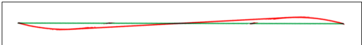
Figure 3.13. Example - Continuous Dubins being longer. After rotating the tangent as shown in Figure 3.11 and 3.12, we can compare the lengths of the results section in the Discrete and Continuous case and conclude that the discrete polygonal arcs are shorter as can be seen above
