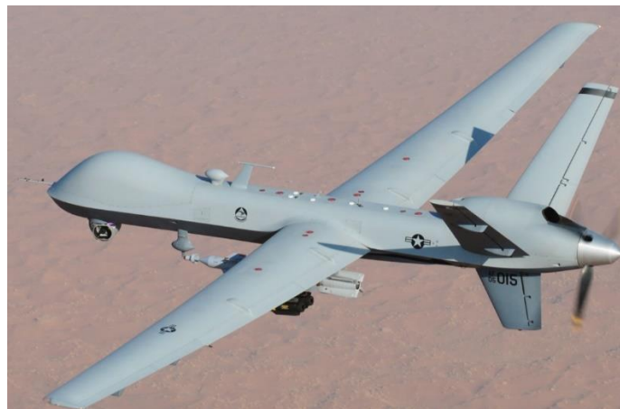
Figure 1.3 U.S. Airforce MQ-9A Reaper Airforce UAV in action. The MQ-9 is the first hunter-killer class UAV designed for long endurance and high-altitude surveillance. It has an endurance of about 42 hours at an altitude of 50,000 feet at max. speed of 250 mph with payload of 3000 pounds. Source: Wikipedia
