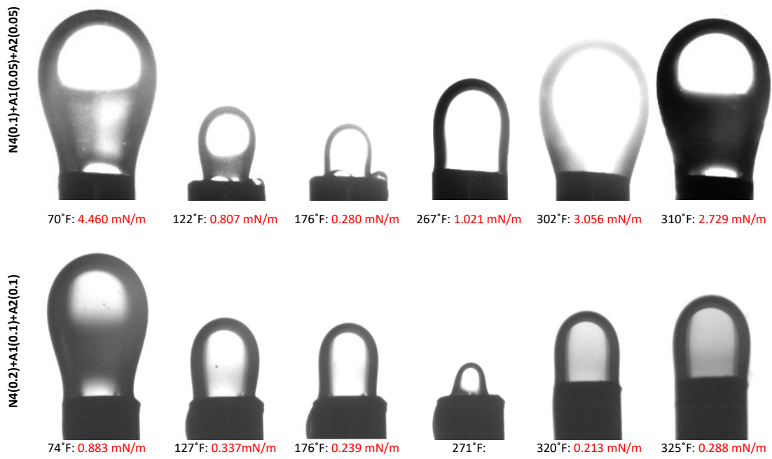
Figure 88: Images of oil drops during IFT experiment using surfactant blends of N4 and A2 in ratio 1:1 showing a decrease in IFT followed by an increase.
