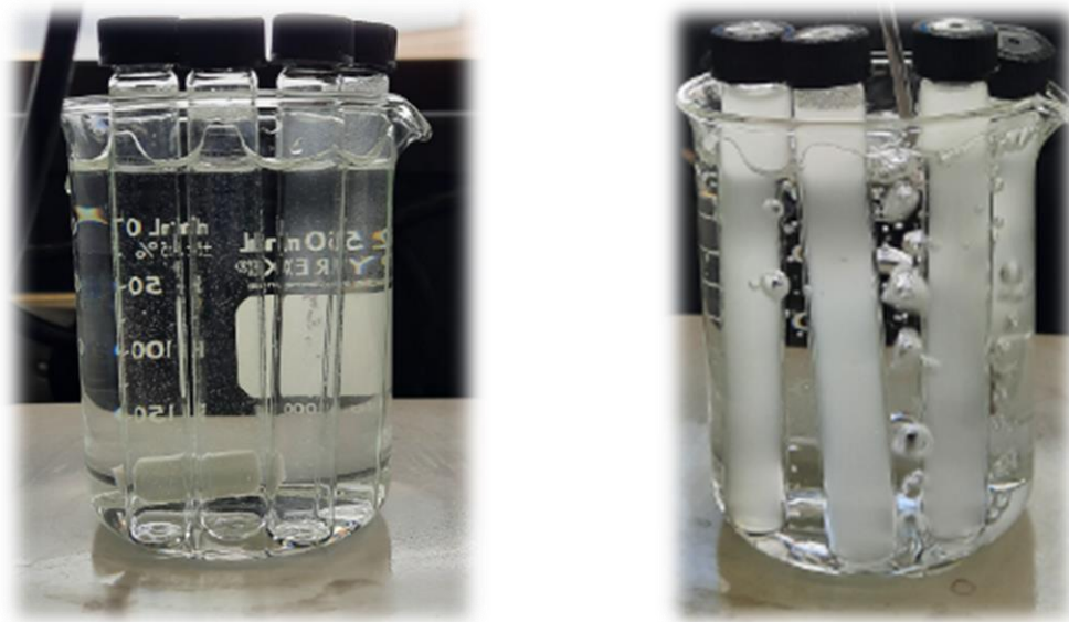
Figure 29: Image of surfactant samples during cloud point tests at low-pressure conditions before heating (left) and above the cloud point (right).
