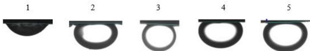
Figure 45: Effect of cosurfactant as thermal stabilizer A3 on contact angles measured on S2 chips at 170°F. Note: Base represents the contact angle after the aging 125.3° (oil-wet). Numbers 1 to 5 represent the sequence in the bar chart. Surfactant blends with anionic co-surfactant A3 produced water-wet CAs.
