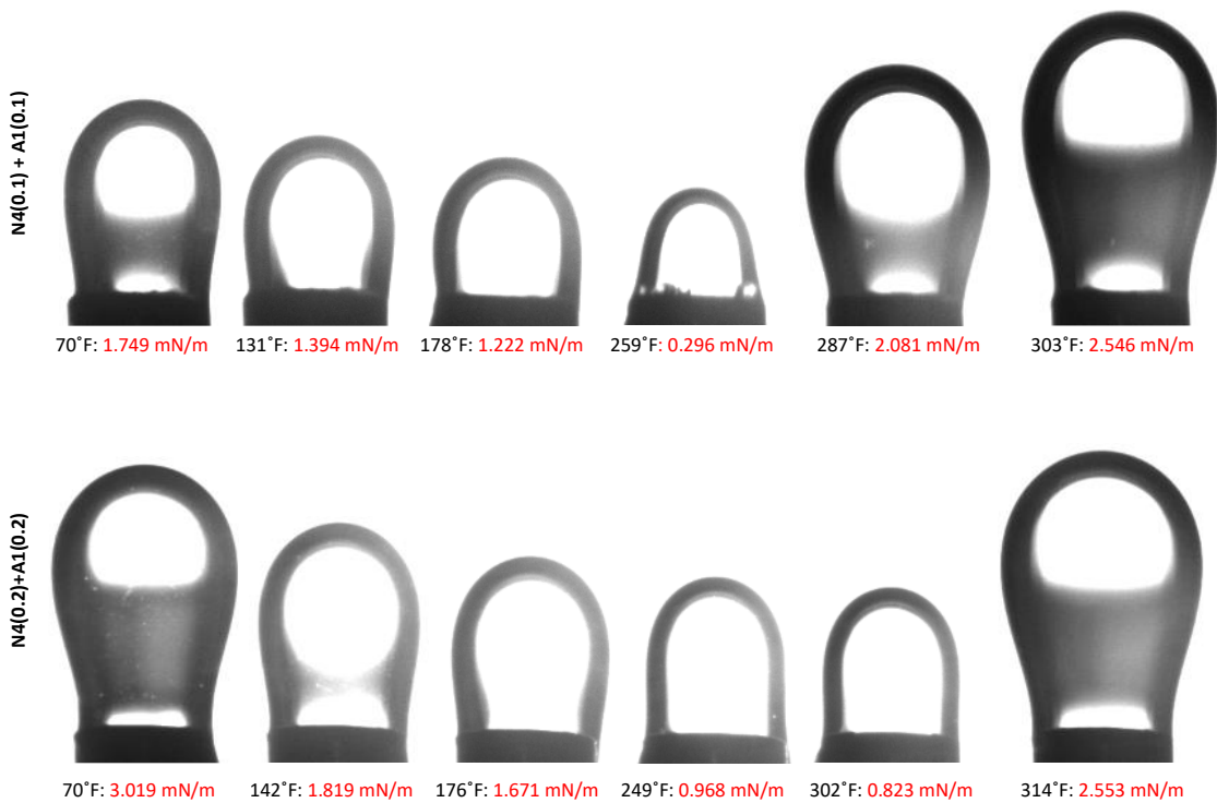
Figure 85: Images of oil drops during IFT experiment using surfactant blends of N4 and A1 in ratio 1:1 showing a decrease in IFT followed by an increase.
