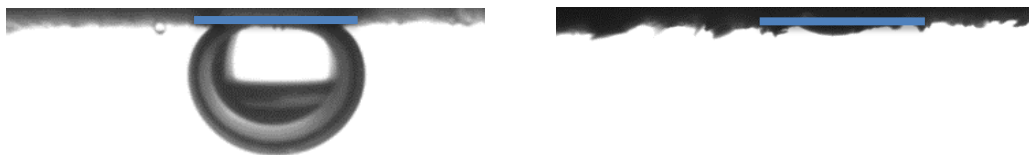
Figure 59: Images of the rock surface at the start of experiment(left) and at the end (right) in N4 (0.4 wt%) + C3 (0.2 wt%) showing degradation of the rock surface.
