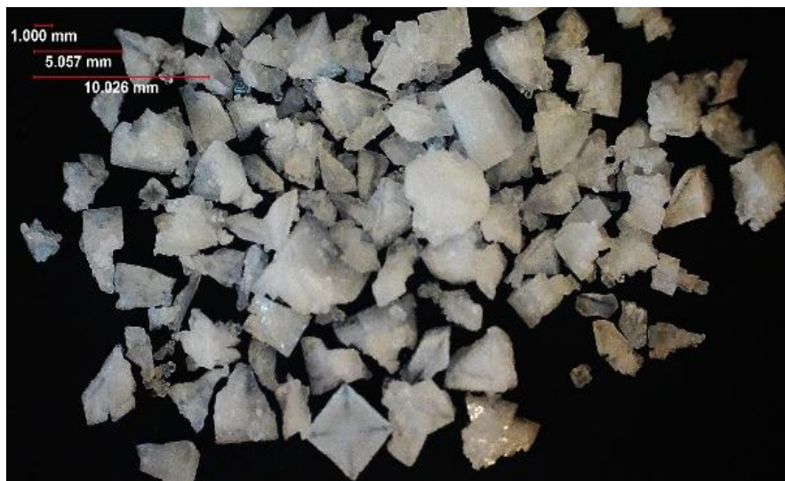
Figure 3.35: A 1.4400g precipitated crystals collected from a 500ppm Trinohex Ultra solution.
