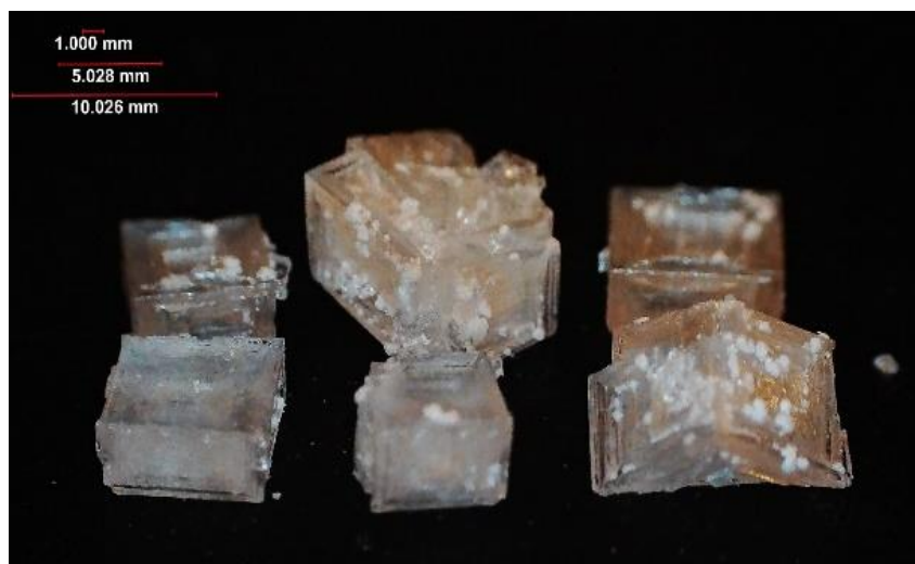
Figure 3.33: A 1.1500g precipitated crystals collected from a 500ppm DMSO solution.
