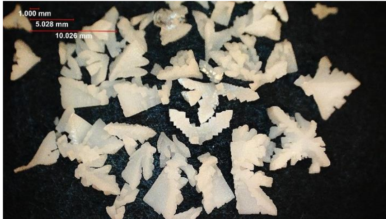
Figure 3.39: Precipitate crystals collected from a 100ppm NTAA solution.
