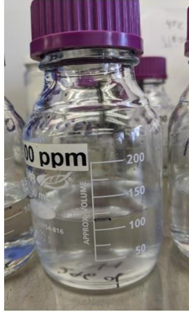
Figure 3.11: 500ppm silica inhibitor bottle after cooling down for 36 hours at 23°C. No precipitate crystals observed.
