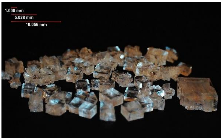
Figure 3.37: A 1.5600g of precipitate crystals collected from a 500ppm TREN solution.
