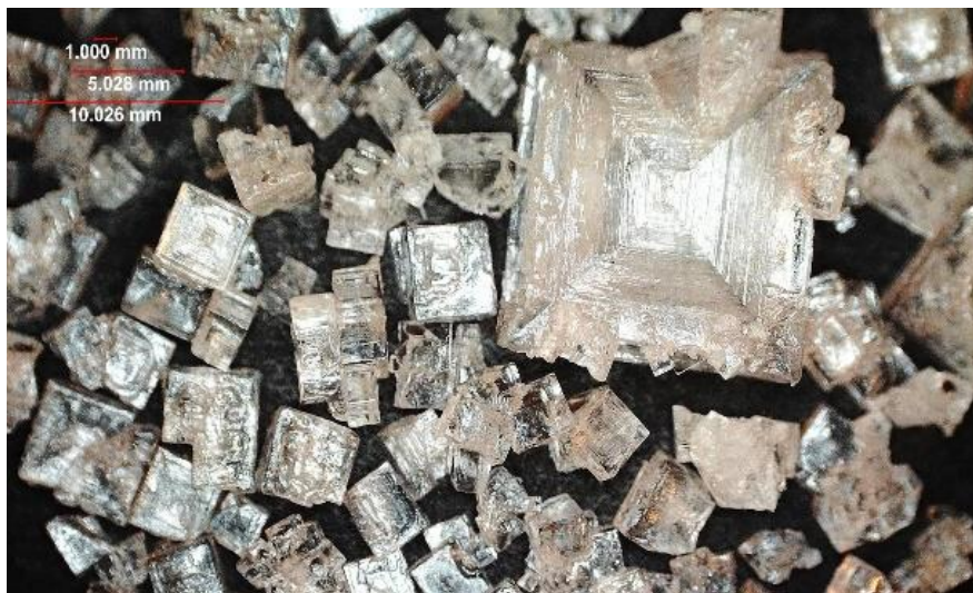
Figure 3.31: Precipitated crystals collected from a 500ppm Dien solution.
