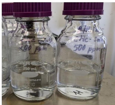
Figure 3.4: 200ppm and 500ppm CMC-Na bottles after cooling down for 36 hours at 23°C.
