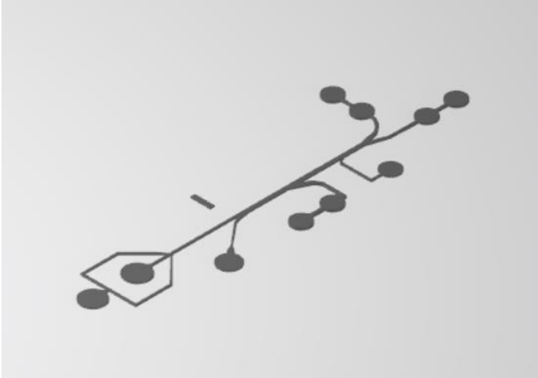
Fig. A.14 (Chapter 7) 2PP printing master mold design for droplet bandpass filter device.
