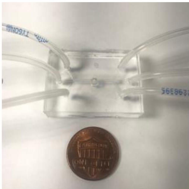
Figure 6 A photo image of the assembled microfluidic platform with tubing.
