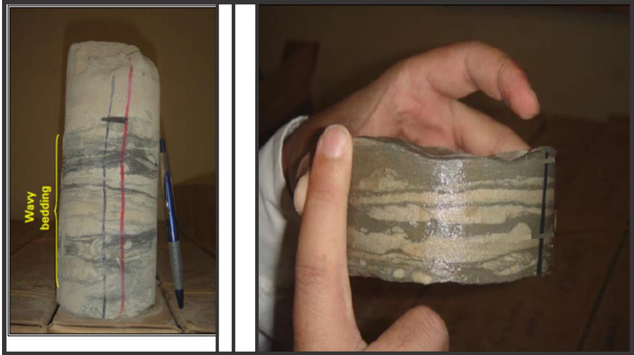
Figure 3.7: Core showing two shale – sand depositional cycles and examples of cross-bedding from cores. On the left image, the first depositional cycle begins with the lower dark distorted shale layer and middle light sand layer. It ends below the upper dark, distorted shale layer. The second depositional cycle includes the upper dark distorted shale layer and the overlying light sand layer. Wavy to flaser cross-bedding types occur in some wells in the study area.
