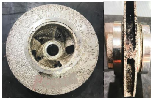
Hastelloy C Impeller [Existing cast] with server pitting corrosion
