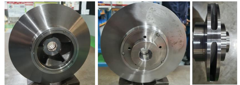
Titanium (Ti6Al4v) 3D printed impeller in service since Dec 2019
