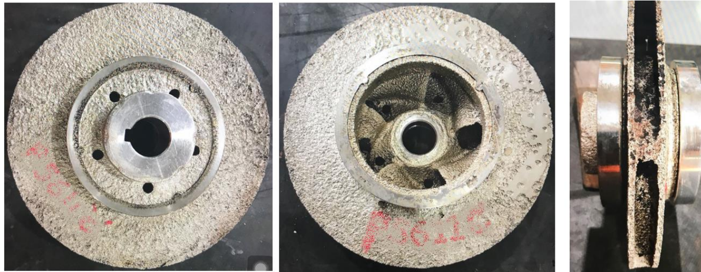
Pitting Corrosion attack on Metal impeller attacked by Sodium Hypochlorite
