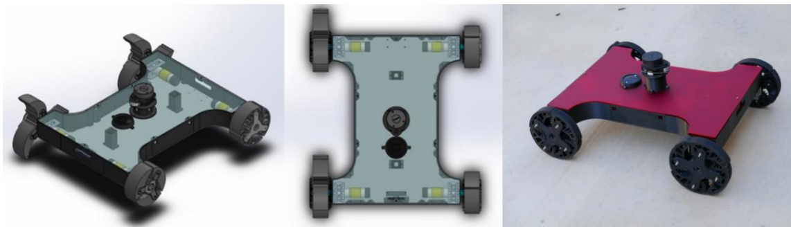
Figure 17. CAD of the chassis (left), assembled prototype (right)
