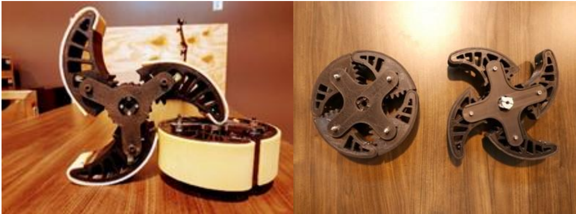
Figure 14. Fully assembled spring-loaded wheel with 3-legs (left) and 4-legs (right)
