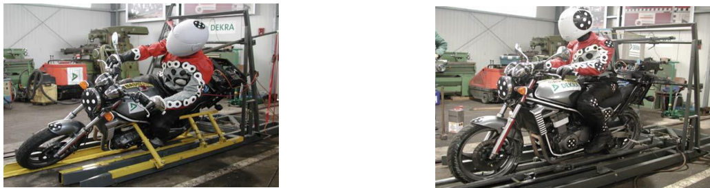
Figure 2.5 Test Sled in (a) Inclined Position and (b) Upright Position (Reprinted from Peldschus et al.,2007)
