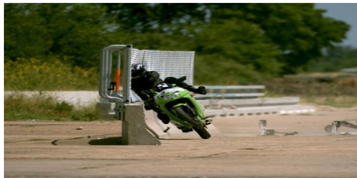
Figure 2.8 Crash Test Image Showing Rider-Motorcycle Barrier Impact (Reprinted from Dobrovlny et al., 2018).
