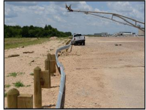
Figure 5.3 Guardrail System with Test Vehicle After Testing (Reprinted from Kovar et al., 2019).
