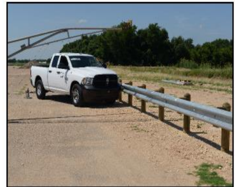
Figure 5.2 Guardrail System with Test Vehicle Before Testing (Reprinted from Kovar et al., 2019).
