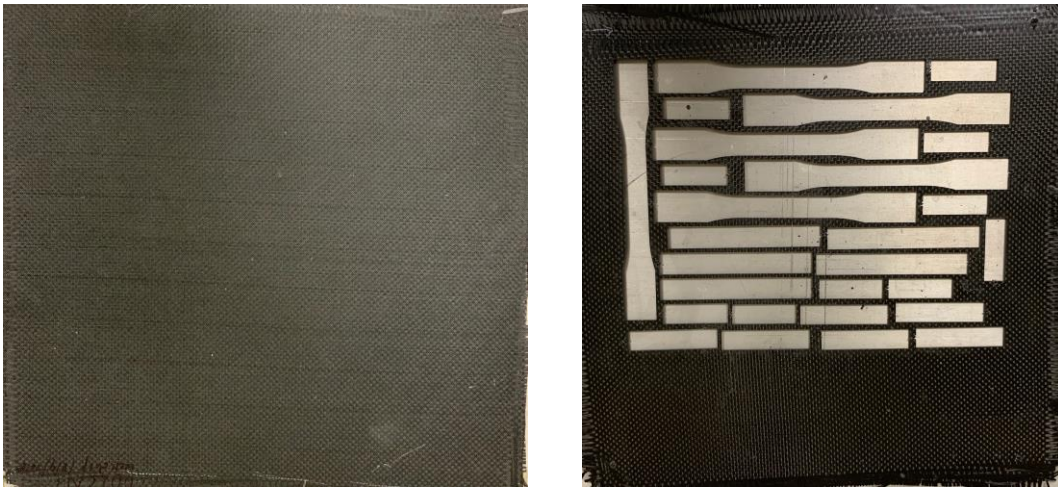
Figure 2.6 Manufactured plates before and after waterjet cutting
