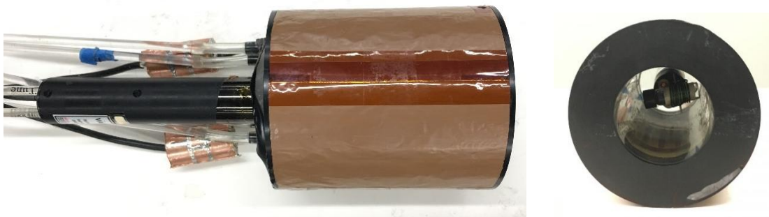
Figure 12. A 6 cm birdcage coil used for ^1\text{H} acquisition (left). An eight-turn solenoid coil with a diameter of 1.5 cm was used for ^{23}\text{Na} acquisition placed inside of the birdcage coil (right). A 5 ml tube filled with 0.6 % NaCl solution was used as a reference phantom.
