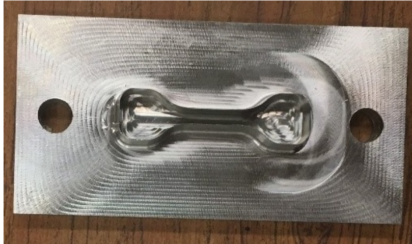
Figure 3.13: Cutmold for specimens in Group 3 and 4
