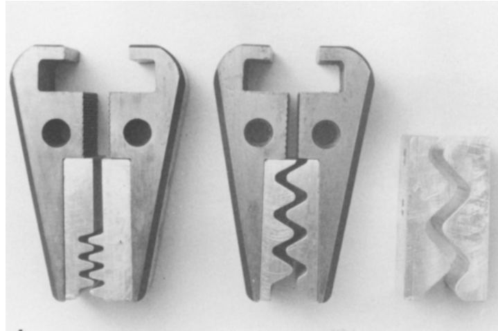
Figure 3.1: Butler's metal serrated clamps, reprinted with permission from [1]
