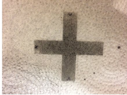
Figure 2.3: Cruciform specimen (painted with speckle pattern)
