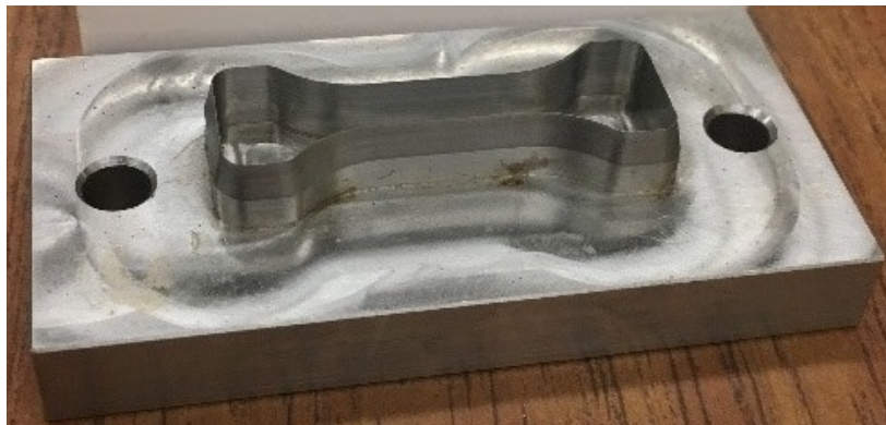
Figure 3.12: Cutmold for specimens in Group 2
