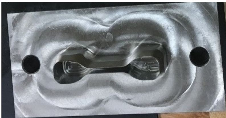
Figure 3.11: Cutmold for specimens in Group 1
