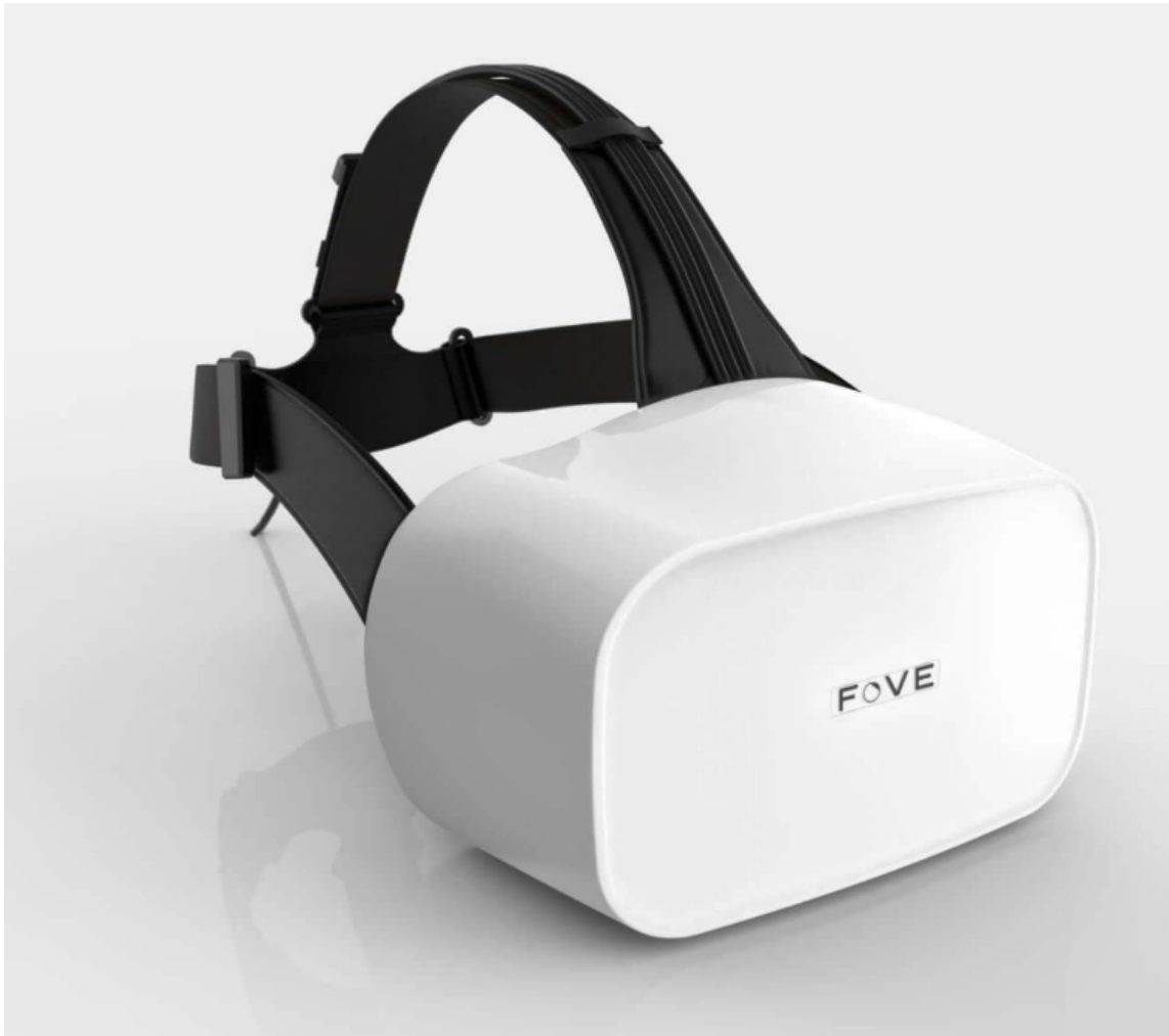
Figure 1.3: FOVE headset with inbuilt eye tracker. Reprinted from [3]
