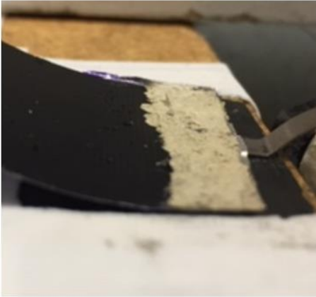
Figure 8. In-situ bimetal-TCSC movement. (a) Heat source in OFF condition. (b) Heat source in ON condition.
