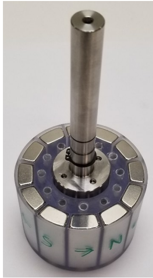
Figure 8.10 Rotor 1 PMs placed in the original Rotor 1 plastic core, which was attached to the high speed shaft.
