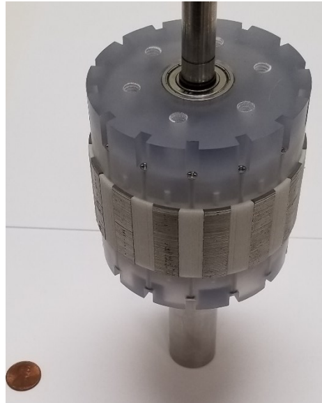
Figure 8.13 Rotor 2 placed around Rotor 1 with a penny provided for a size reference.
