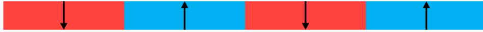
Figure 7.1 Conventional surface permanent magnet magnetization arrangement, which is equivalent to a discrete Halbach array with one segment per pole.
