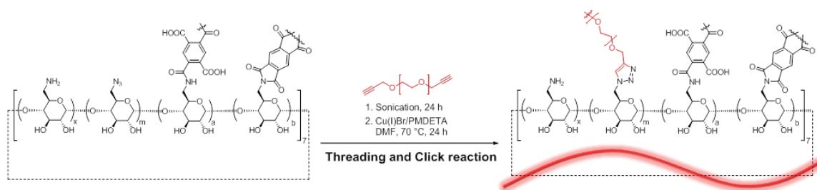
Figure V.3. Synthesis of slide-ring CDPI gels, in which linear poly(ethylene oxide) (red) is threaded through the cavity of the cyclodextrin before immobilization by cross-linking.
